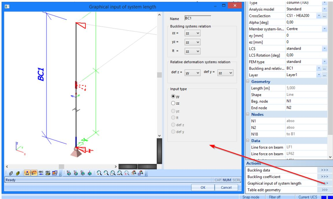
When the buckling parameters are set, you can continue with the steel check. Before you proceed deactivate the **System lengths** and **Local axes** representation by means of the **Fast adjustment of viewflags on whole model**
