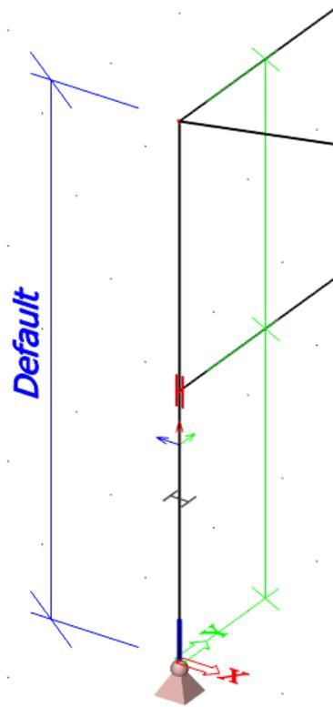
The figure shows that (default) system length  $L_y$  (blue line) for buckling around the strong axis (y-y) is total height of the column and  $L_z$  (green line) for buckling around the weak axis (z-z) is half of the height. The girder in the middle of the column therefore supports the column for buckling around the weak axis, i.e. for bending in the Y direction.
