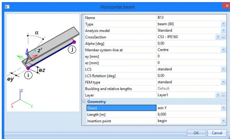
3. As the structure type **Frame XYZ** has got two horizontal axes (i.e. X and Y), you must indicate the right direction for the horizontal beam in the **Direct** field. Choose **axis Y** possibility.
