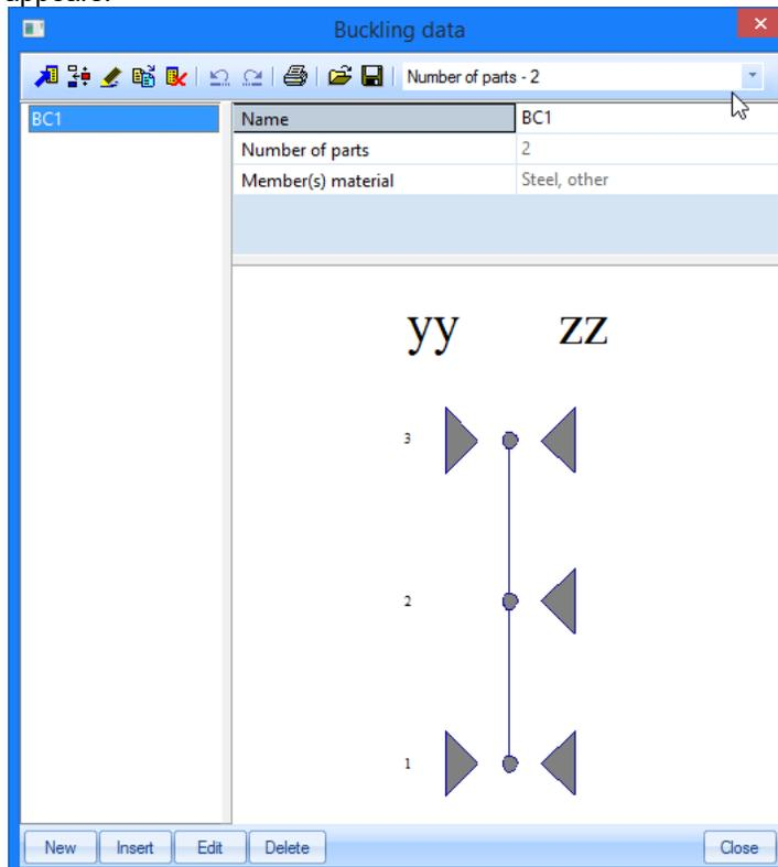
This window shows that the column is supported for buckling around the weak axis (zz) in the middle and that it is not supported for buckling around the strong axis (yy) in the middle – the grey triangle is missing on left hand side.
