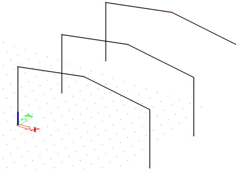
Connecting beams of the frames can be entered when the frames are entered. The start and end nodes of the beams are already known, i.e. begin and end nodes of the entered members. Therefore you do not have to enter the beams by means of coordinates; instead of that you can use the **Cursor snap settings**.
