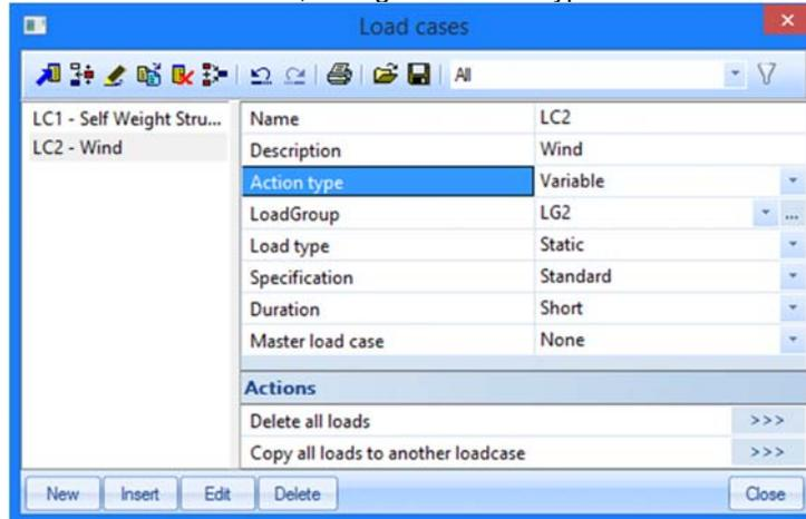
4. The Load Group LG2 is automatically created. Click
