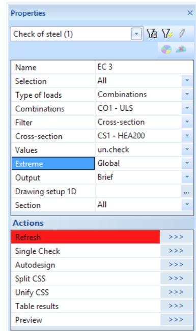
3. In the **Property** window, click the **>>>** button next to **Refresh** to display the results in the graphical screen in accordance with the above parameters.
