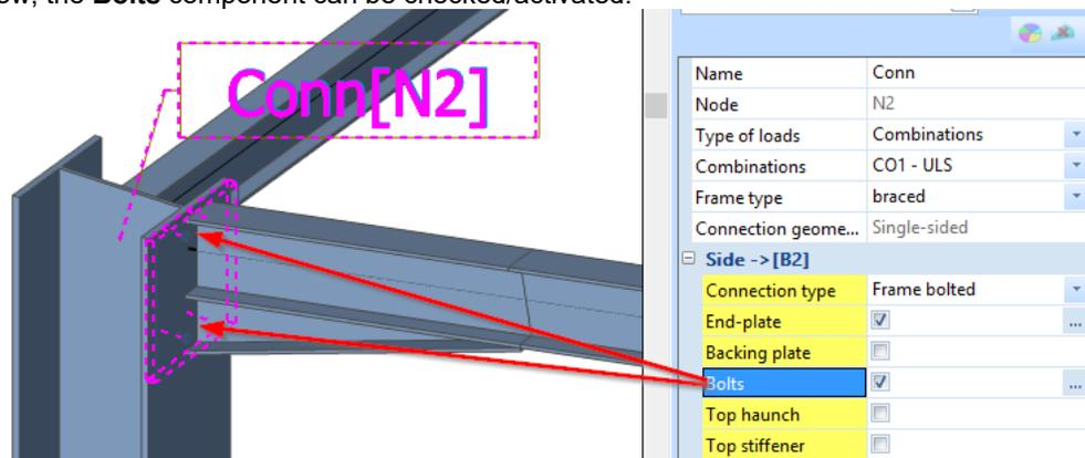
The bolts are automatically displayed in the graphical screen.
