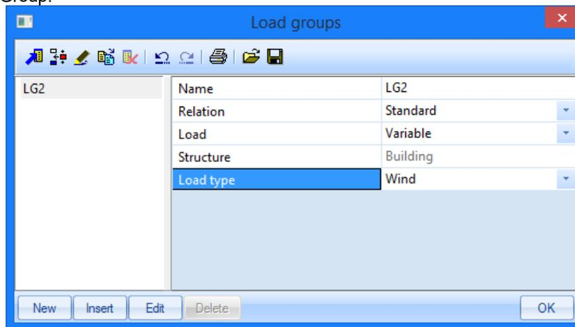
The Load type determines the composition factors that are attributed to the load cases in this load group. In this project choose **Wind**.
