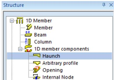
2. As indicated, a haunch requires a cross-section with a possibility to create variable dimension(s). Since this project does not contain any variable profiles yet, the **New cross-section** window automatically appears.
