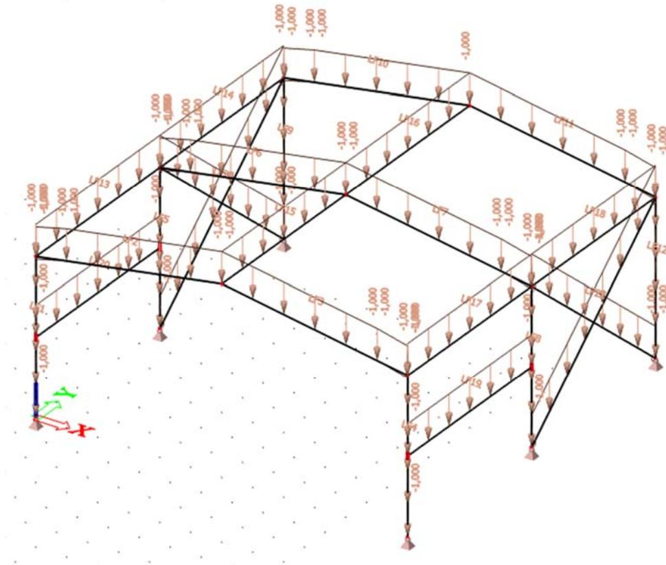
Next, the roof weight is entered as a surface load of 1,5 kN/m<sup>2</sup>. Only the roof girders are loaded directly.
