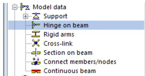
2. The hinges are put to both ends of the diagonals; therefore choose **Both** for the **Position** when dialogue **Hinge on beam** pops-up.
