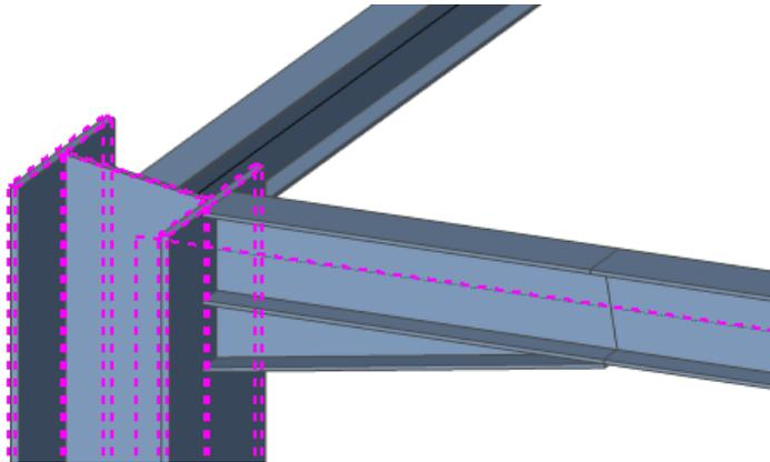
5. Press **<Esc>** to finish the selection. Connection is inserted (by the mean of a flag named Conn1) and the properties, including components, are displayed in the **Properties** window.
