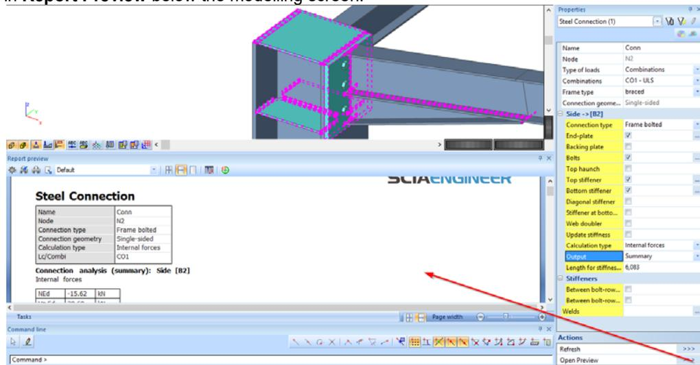
Output shows the internal forces, design resistances, results of unity checks and moment-rotation diagrams. The most significant part of the output says that this particular connection does not satisfy the check, therefore we have to change the configuration of the connections.
