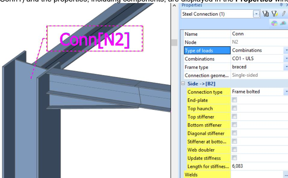
6. Now, the components of the connection can be entered. Activate (check) the **End-plate** option. The end plate is entered and immediately displayed in the graphical screen:
