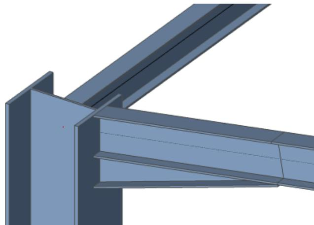
The structural model shows the structure as it will be realized in practice. On this model, you can introduce the connection because now its position is fully clear.
