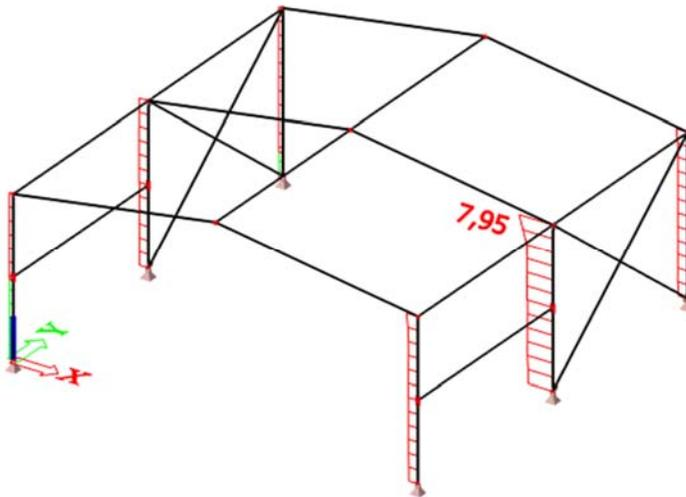
Graphical screen shows that the maximum unity check occurs for one of the middle columns. To understand the reason behind you can open the **Report preview** with a detailed representation of the performed steel check. You can find all input data, calculated resistances, code formulas and notices and warnings in the detailed output that usually contains a few A4 pages.
