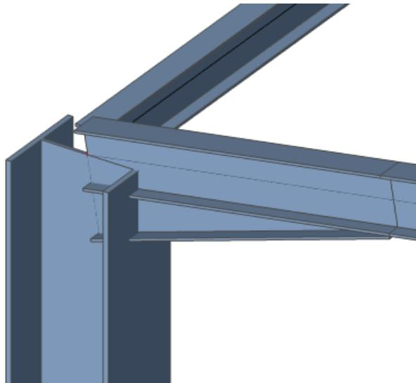
3. In this analysis model, the bars are arriving in the same node, i.e. node **N2**. But in practice the girder is cut for instance at the column flange or vice versa. In SCIA Engineer, you can indicate this through the structural model.
