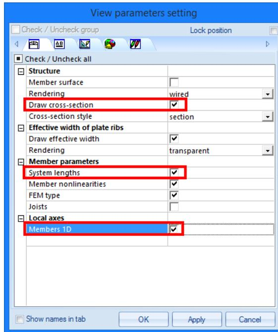
4. Activate the **System lengths** and **Draw cross-section** options to display the reference lengths and the section of the bar.
