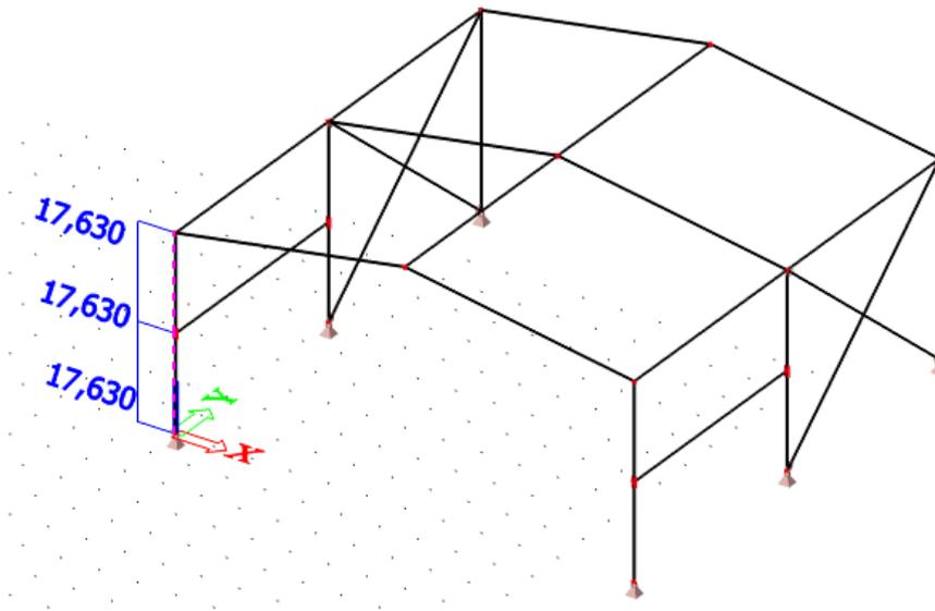
The buckling length is determined as reference length **Ly** multiplied by buckling factor **ky**.
