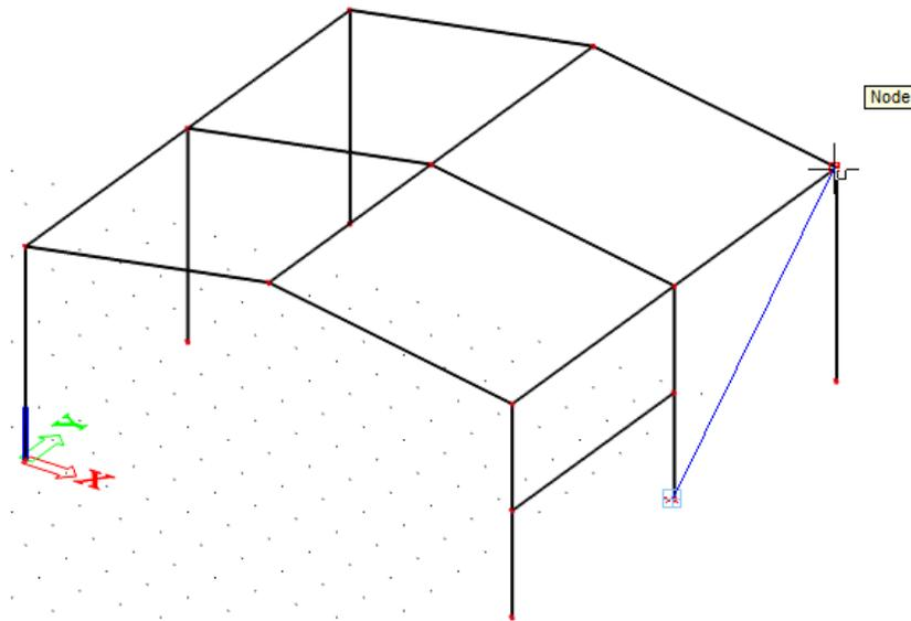
6. Repeat selecting start nodes and end nodes until all bracings are modelled.
