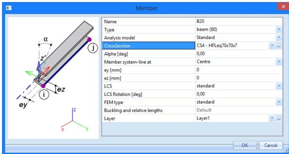
2. In the **Type** field, choose **Wall Bracing (0)**. This specification is considered for the STRUCTURAL model only and does not influence the calculation model or the results.
