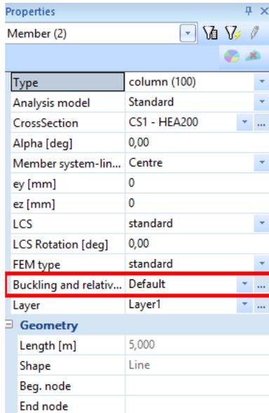
3. Click the **...** icon next to **Buckling and relative lengths**. The **Buckling data** window appears.
