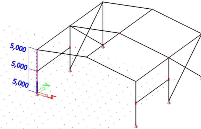
As already indicated in the buckling parameters, the reference length is 5m.
