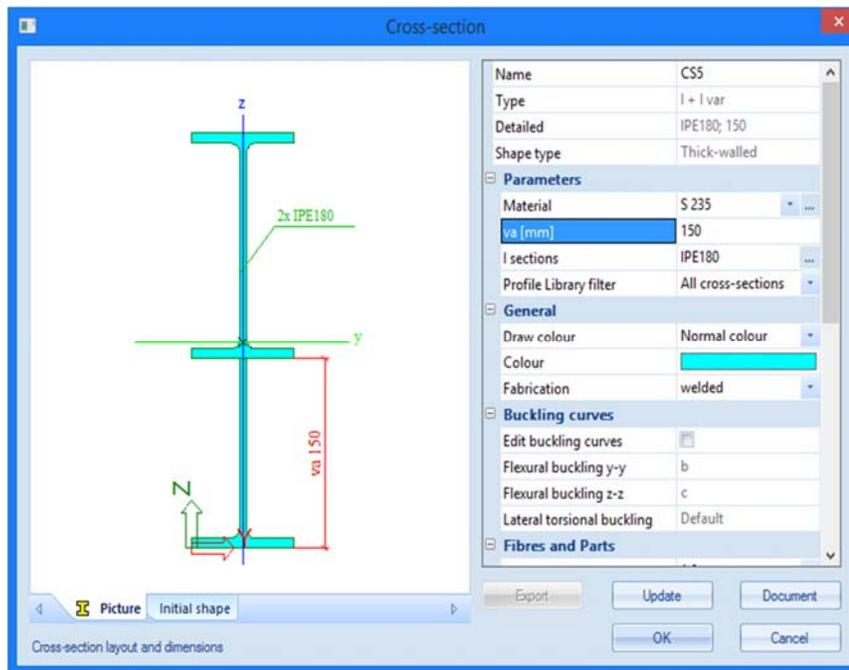
6. In the **I sections** field, change the section in an **IPE 180** by clicking the **...** button behind the section type.
