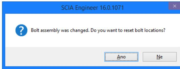
Click **Yes**: the bolt positions, intermediate distances, edge distances etc. are automatically adapted to the new bolt type.
