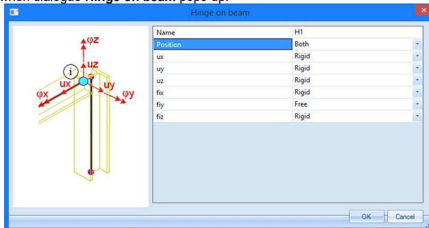
3. To obtain a hinge, the rotation **fiy** is set to **Free**, the translations and the other rotations remain **Rigid**. In this way, the diagonals will be exclusively hinged in the planes of the sidewalls.
