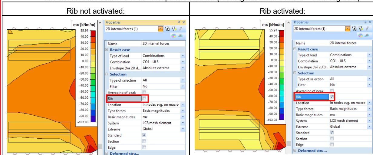
2. Note the difference for the two ribs that are modelled. It is clear that the forces in the plate are reduced, because the joint stiffness of the slab and the ribs is now considered.
