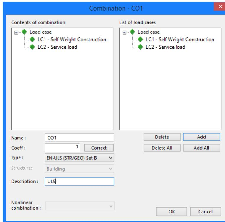
3. The Type of the combination is changed to **EN – ULS (STR/GEO) Set B**. With this envelope combination type SCIA Engineer will automatically generate linear combinations in accordance with the complex composition rules of the Eurocode.
