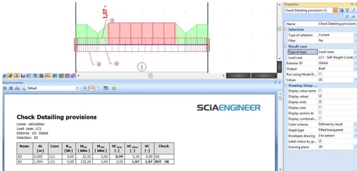
5. Shear reinforcement check shows value higher than 1,00 at particular span. We need to shorten the distance of stirrups to satisfy the detailing provisions.
