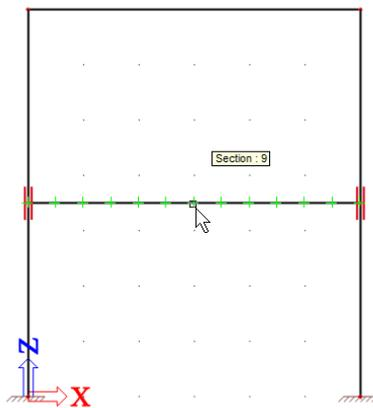
4. A new dialogue **Section check** opens. Here you can define reinforcement template in that particular section, edit diameter and number of bars and directly see the unity check value. Number 3,00 with the red cross means that the current reinforcement does not satisfy.
