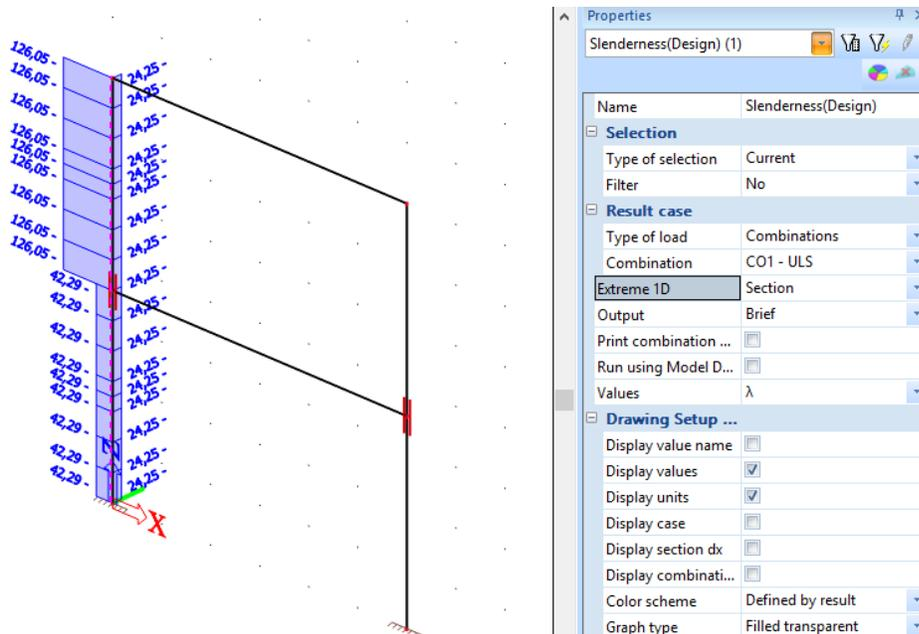
4. Change the **Values** field to **I** to display the buckling length for buckling around both axes. Hit again the **Refresh** action button to regenerate the view.
