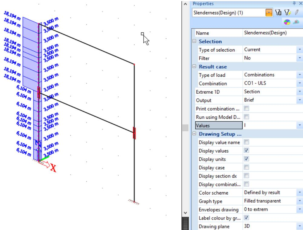
As already indicated in the buckling parameters, the buckling length is 3,5 m.
