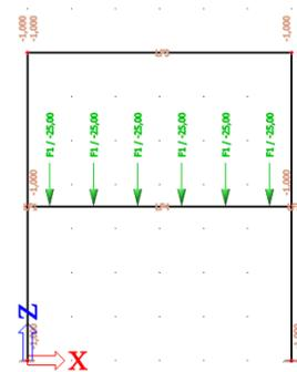
The roof beam is similarly loaded with concentrated loads of **12.5 kN**. Therefore, the load of the floor beam can be copied to the roof beam and adapted according to the steps below.
