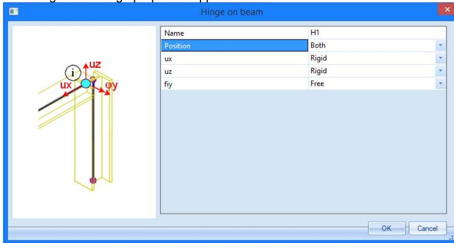
3. The hinges are entered on both sides of the beams, so that you have to choose **Both** for **Position**.
