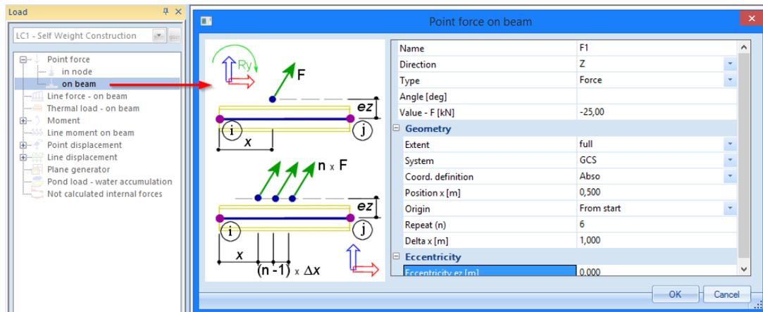
2. The floor beam is charged with 6 concentrated loads of **25 kN** with a distance of **1 m**. The first concentrated load of the series is at **0.5 m** from the starting node of the beam.
