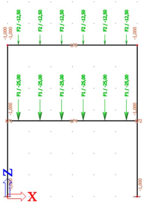
After input of the loads in the first load case you can enter the service load into the second one. The floor beam is loaded with a service load of 10 kN/m.
