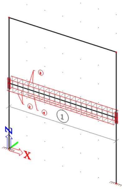
After the input of practical reinforcement layers, these layers are additional data on beam. They can be copied easily to other beams.
