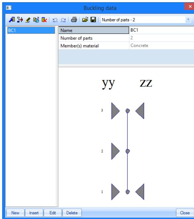
This window shows that the column is supported in the middle for buckling around the strong axis (Y-Y) but not for buckling around the weak axis (Z-Z).
