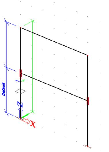
The figure shows that system length ( $L_y$ ) for buckling around the strong axis (y-y) is 3,5 m and  $L_z$  for buckling around the weak axis (z-z) is 7 m. The beam in the middle of the column therefore supports the column for buckling around the strong axis.
