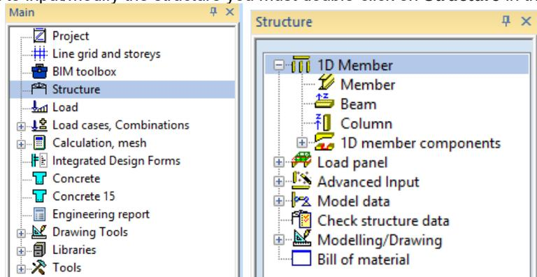
2. In the **Structure menu**, you can choose different structural elements to enter the structure.
