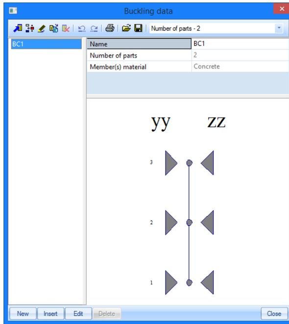
9. The **Properties window** indicates that the buckling parameter **BC1** is used for both columns.
