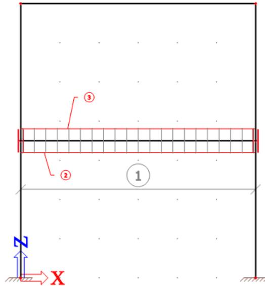
6. We have calculated that some additional reinforcement was required in the middle of this beam. Therefore we will add a new bar of reinforcement in the zone from 1 m to 5 m.
