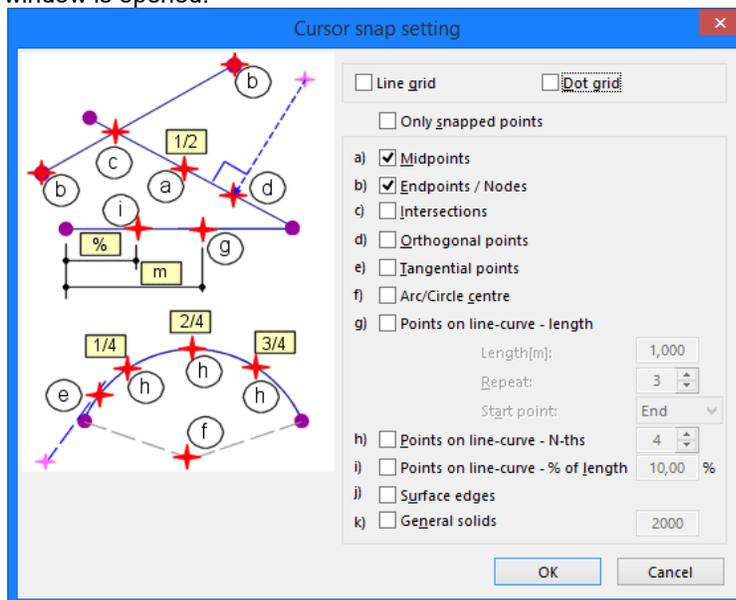
2. Activate the options **a) Midpoints** and **b) Endpoints/Nodes** to pick the desired locations on members in this project.
