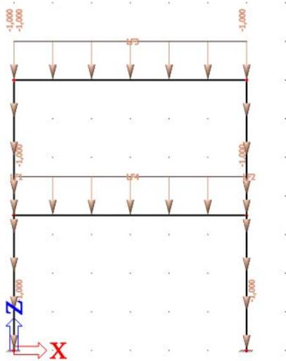
Now, the floor and roof weight is entered as a series of concentrated loads:
