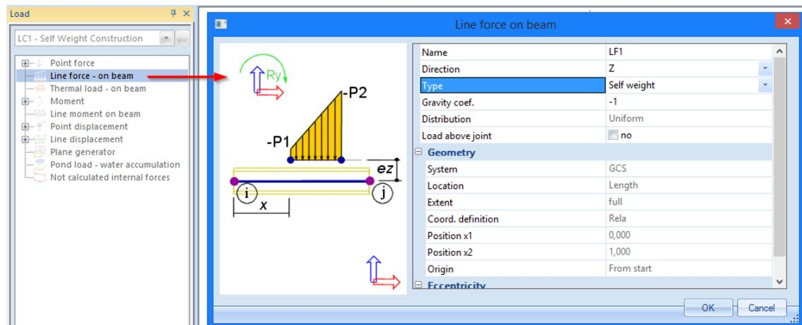
3. In the field **Type**, choose **Self Weight**. The **Direction** is the global Z-direction and the **Gravity coefficient** is set to **-1**, so that the load is acting vertically downwards.
