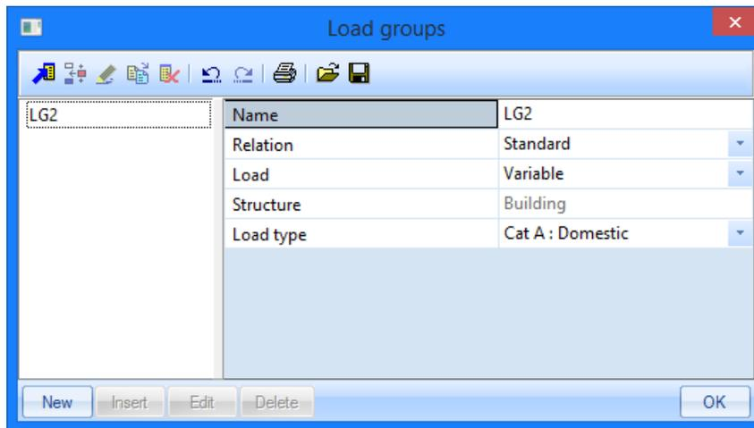
The Load type determines the composition factors that are attributed to the load cases in this load group when Eurocode combination is requested. In this project, choose **Cat A: Domestic**.
