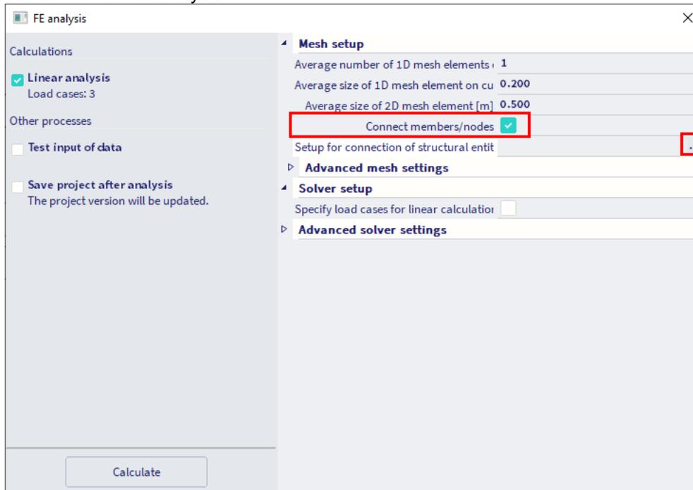
Click on the three dots next to **Setup for connection of structural entities** to open the dialogue with the settings. Activate the option **Connect 1D members as ribs**. This option will connect the plate and the beams as a rib.
