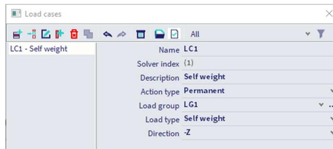
We will create a second permanent load case for the roof weight. Click on **[New]** and change the **Description** to **Permanent**. The **Load type** is now set to **Standard**.
