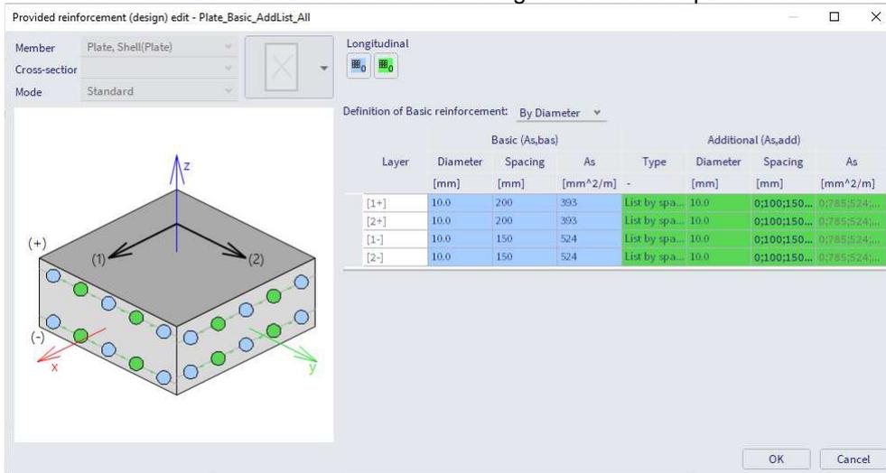
You can add practical or user reinforcement to the 2D member(s) via 2D reinforcement in workstation Concrete of the process toolbar (or via the input panel).
