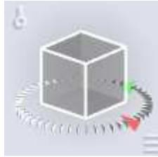
You can rotate/tumble, pan, zoom, set the view in the direction of one of the global axes,... All possibilities are shown on following help-page:
