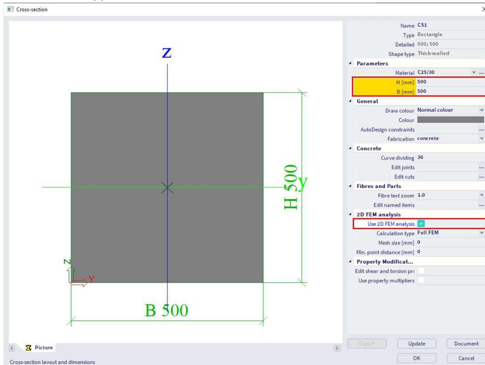
Set **H** as **500 mm** and **B** as **500 mm** and activate the option 'Use 2D FEM analysis' (in order to calculate the torsion and warping properties correctly). Click **[OK]** to confirm, the cross-section is now added to the cross-section list in your project. Add another rectangular cross-section with **H = 700 mm** and **B = 450 mm** in a similar way.
