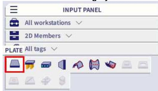
Via **ALT and right-mouse click** you can also use the **Marking menu** to quickly launch the Plate command in the Model tab.
