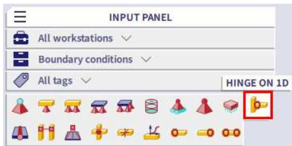
The hinges are put to both ends of the diagonals; therefore choose **Both** for the **Position** when dialogue **Hinge on beam** pops-up.
