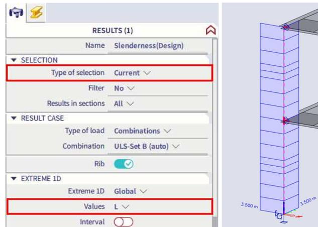
You can ask as well for the slenderness ( $\lambda$ ), buckling factor ( $\beta$ ), buckling length ( $l$ ), ... The buckling length is determined as the reference length multiplied by the buckling factor.
