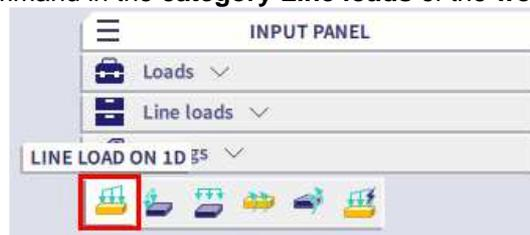
Set **Value - P [kN/m]** to **-1.00** in the properties dialogue. The load **Direction** is **Z** and the **System** is the local coordinate system **LCS**. The linear loads are acting in accordance with the local Z-axes of the elements.
