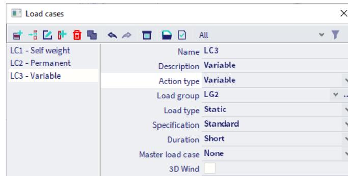
The **Load type** determines the composition factors (psi-factors) that are attributed to the load cases in this load group. There are different categories available, as well as Snow, Wind, ... In this project choose **Cat A: Domestic**.
