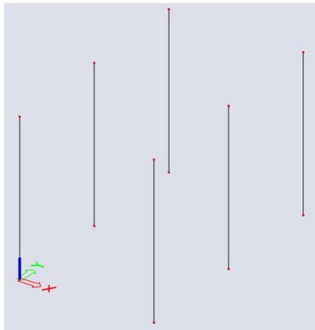
*Note:* it's possible to connect the frames automatically with beams with the multicopy command. Therefore use the option **Connect selected nodes with new beams**. After confirming with **[OK]** the software will ask you for the cross-section for the new beams. When you use this option for your structure, you don't need to select the lower nodes of the columns in this case.
