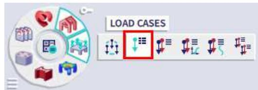
Before you can define loads, you must enter load cases first. Since this project does not contain any load cases yet, the **Load Cases** manager will automatically appear and by default, the load case LC1 is automatically created. This load is a permanent load of the **Self weight** load type. The self weight of the structure is automatically calculated, although not graphically displayed.
