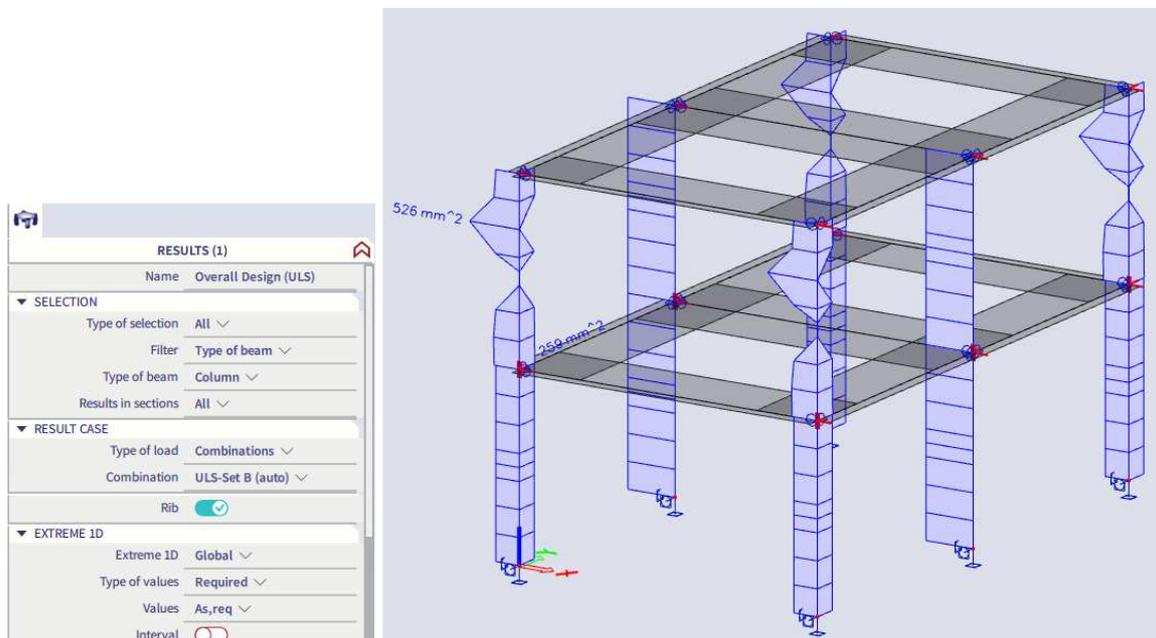
It is also possible to show the provided reinforcement. (Type of values = Provided). This will give you a proposal based on the **Design defaults** you have set for the column in the **Concrete settings**.
