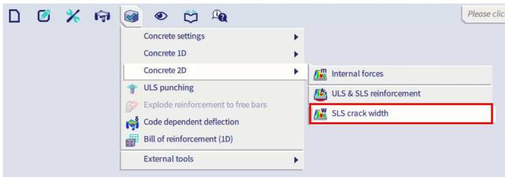
Finally, you can execute the code dependent deflection check with the required reinforcement, provided reinforcement or user reinforcement. This check will take into account long-term effects such as creep and shrinkage.
