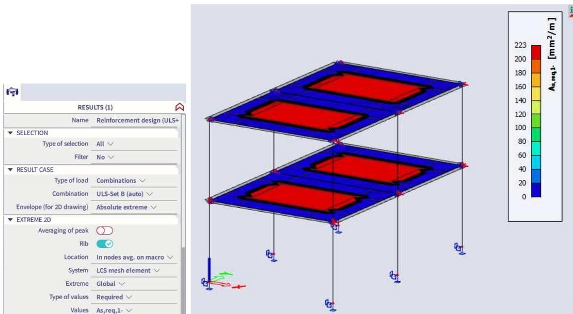
In the view settings you can activate the Drawing directions for design, so it's clear what is direction 1+, 1-, 2+ and 2-:
