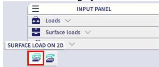
Set **Value [kN/m<sup>2</sup>]** to **-2.50** in the properties dialogue. The **Direction** is the global **Z** direction and the value is negative, so the load is acting vertically downwards.
