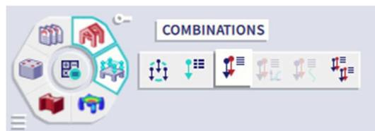
Three code combinations are created, one for the Ultimate Limit State and two for the Serviceability Limit State (characteristic and quasi-permanent).
