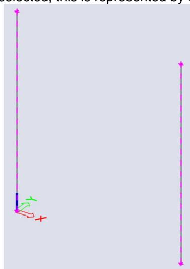
Now, you can select the **Multicopy** command via **Main menu > Edit > Modify > Multicopy** or with the icon in the **workstation Structure** or with the icon in the Modify tab of the **Marking menu**. In the **Number of copies** field enter **2**. To manually set the distance between the frames, deactivate the **Define distance by cursor** option. Now, you can enter the distance 5 m in direction Y.
