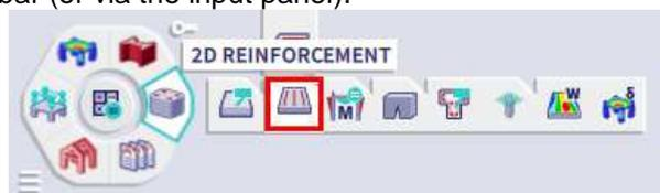
You can execute the reinforcement design including the user reinforcement with the option Consider user reinforcement in the property panel.
