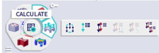
Make sure that the option **Connect members/nodes** is turned on in the **Mesh setup**, so all entities are properly connected before the analysis. Select **Linear analysis** and press **Calculate**.
