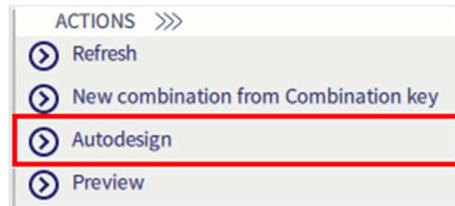
*Note: steel optimization works with cross-sections, not particular members. Therefore once the cross-section is changed, all members with that profile are changes as well. Therefore in the property panel the **Filter** should be set to **Cross-section** when you use the Autodesign action.*
