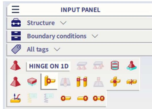
The hinges are put to both ends of the diagonals; therefore choose **Both** for the **Position** when dialogue **Hinge on beam** pops-up.
