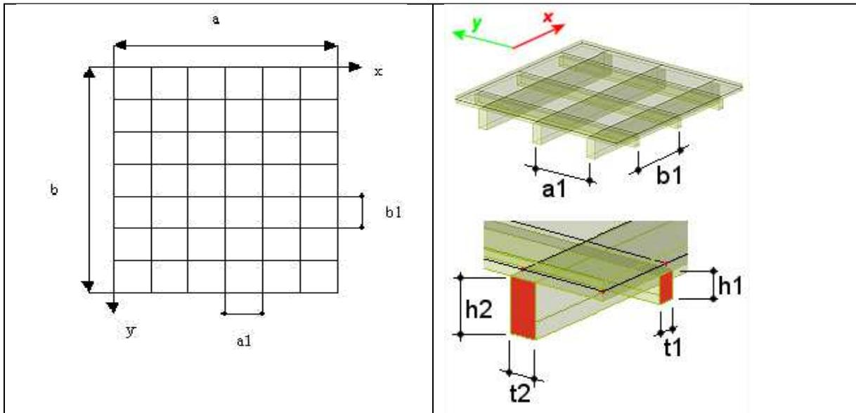
The user must input the rib dimensions, rib spacing and slab height.
