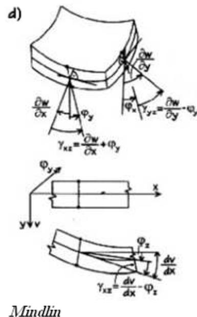
The choice between these two elements can be made using the menu function **Calculation, mesh > Solver setup**. Default the Mindlin theory is used and because of this, special attention has to be paid to the use of thin plates.
