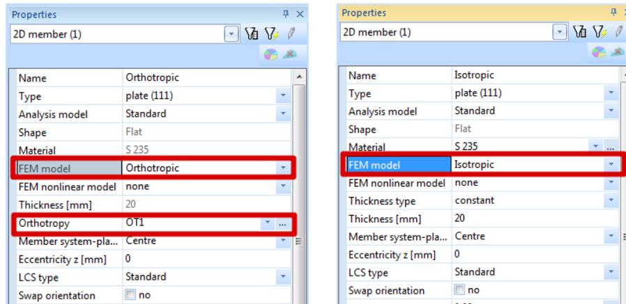
In OT1 (orthotropic properties), the option 2 heights will be chosen. This allows both the flexural and membrane strengths to be configured with height parameters. The '1' direction corresponds to the x-axis of the Local Coordinate System of the plate, the '2' direction corresponds to the y-axis (which can also be derived from the explanatory image below).
