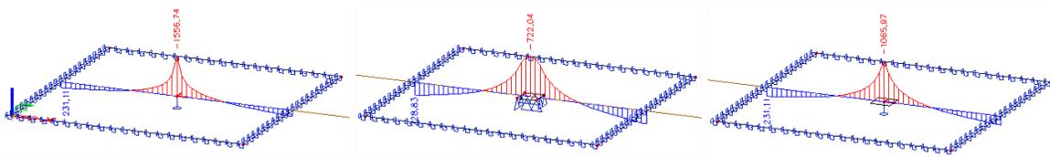
The structure is calculated with Mindlin elements. The results are claimed in nodes, averaging. The table below shows the maximal value of  $m_x$  above the nodal support or the subregion.
