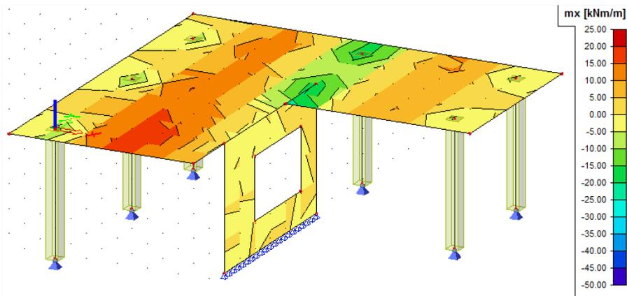
The results are not alike, which means that the post-processing has quite a big impact on the representation of results. This indicates that the mesh is not fine enough.
