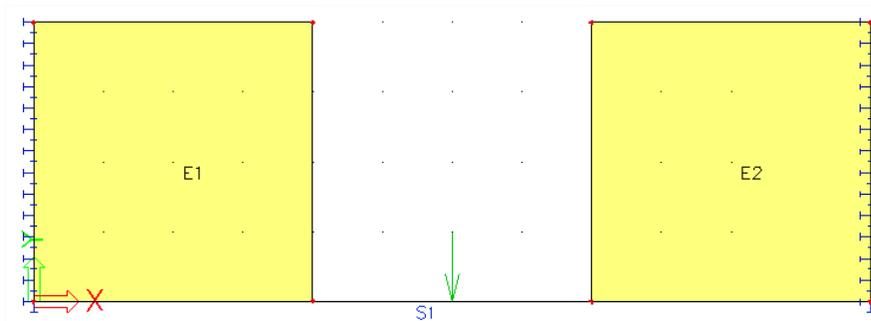
Even though the beam is fixed on both walls, it seems that it has a moment of zero at the connections. In other words, it looks like there are hinged connections. The beam seems to be hinged due to the fact that plates do not have a moment  $m_z$ , since torsion in the plane of a plate is always taken up by the normal forces  $n_x$  and  $n_y$ .
