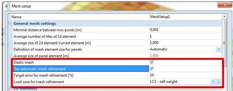
2. Perform the linear calculation. You will also receive information about the error estimation for the load case configured in the previous step.
