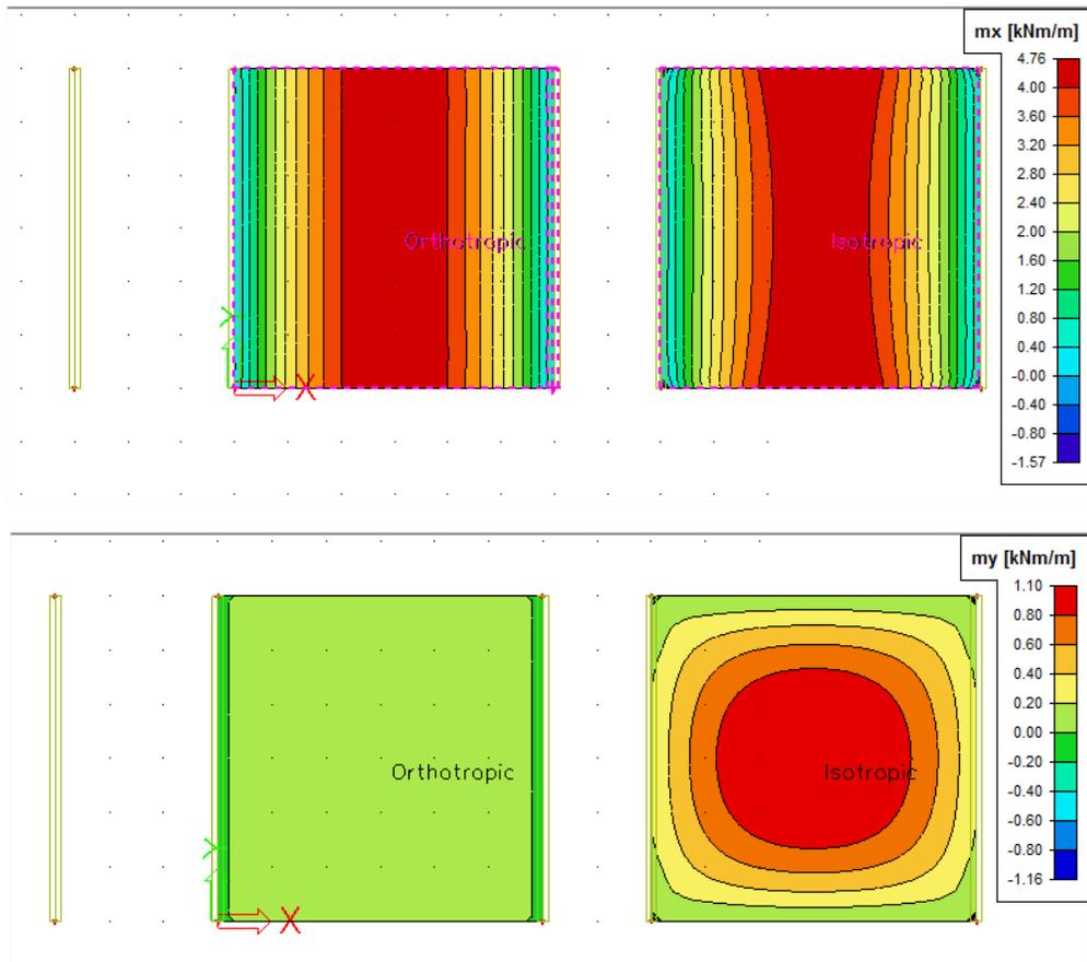
Thus the transverse bending stiffness of the isotropic load reduces the amount of load which would be sent to the beams.
