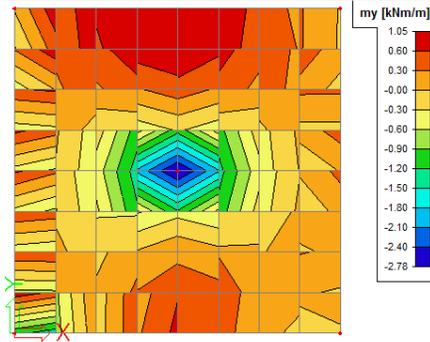
When changing this average strip from perpendicular to longitudinal, an average will be made for  $m_y$  but not anymore for  $m_x$ .
