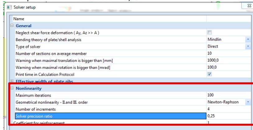
When the calculation is performed, the elements which take tension will have their rigidity reduced in the direction of the tension stress. The rigidity is reduced uniformly in that direction for the entire finite element. For this reason, the mesh must be sufficiently fine (in this example **0,150m** is used).
