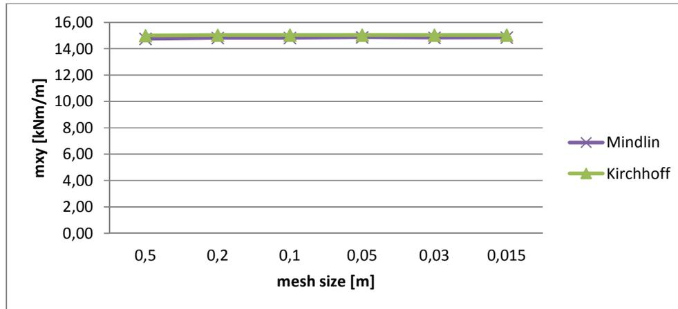
The comparison for the **thick plate** shows that when the calculation is done with Mindlin,  $m_{xy}$  reaches lower values, even with a rougher mesh size (a mesh of 0,5m).
