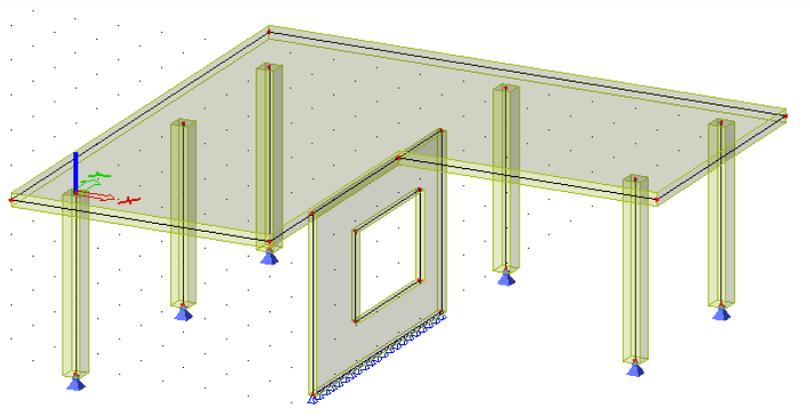
The project start with a mesh size of 1m for the 2D elements.
