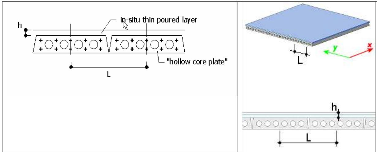
The rigidity in the main direction is calculated based upon the properties of a user defined cross-section. The user should define the cross-section (CSS) of these unidirectional prefab elements and then use this CSS to define the orthotropy.
