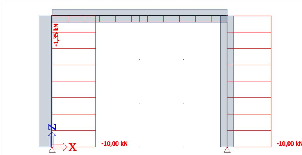
The increased moment on the left column is due to the eccentricity which has been applied. The additional moment can be calculated as:
