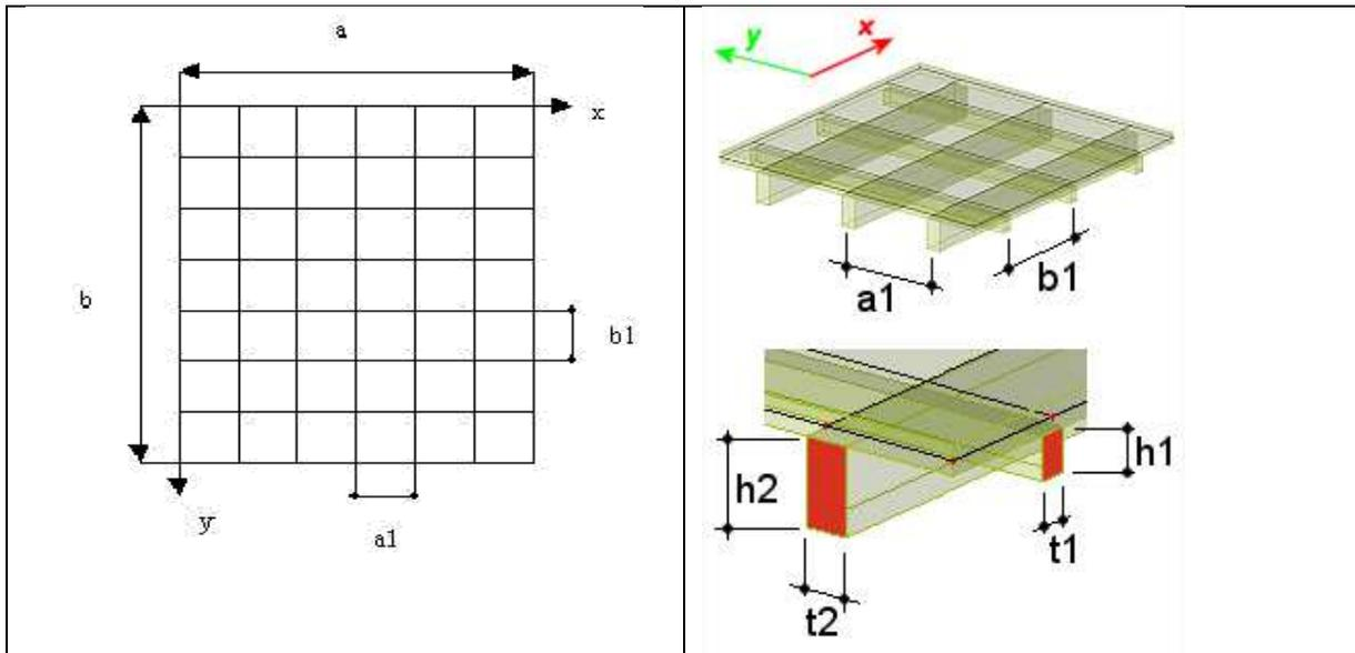
The user must select the ribs from the library and input the rib spacings and slab height.
