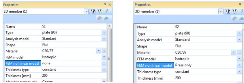
To calculate this non-linear setting, the non-linear calculation must be done. This requires non-linear combinations. Since a non-linear combination is non-associative, loads must be combined before the calculation, as opposed to the linear calculation. And thus non-linear combinations are required.
