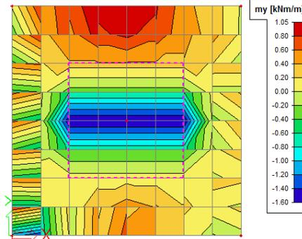
**Note:** The averaging algorithm uses only the finite elements that are located inside the averaging strip.
