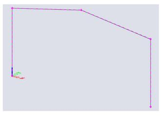
Now, you can select the **Multicopy** command via **Main menu > Edit > Modify > Multicopy** or with the icon in the **workstation Structure**. In the **Number of copies** field enter **2**. To manually set the distance between the frames, deactivate the **Define distance by cursor** option. Now, you can enter the distance 6 m in direction Y.
