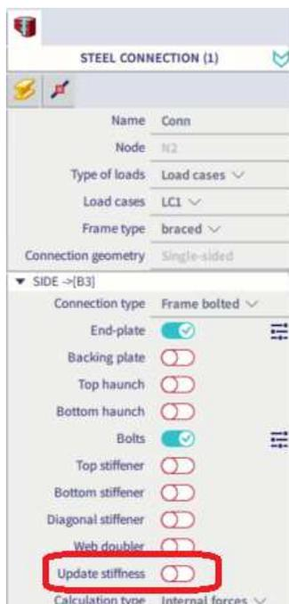
After recalculating the project, a hinge will be added to this connection with this stiffness  $S_{j,ini}/\eta$ .
