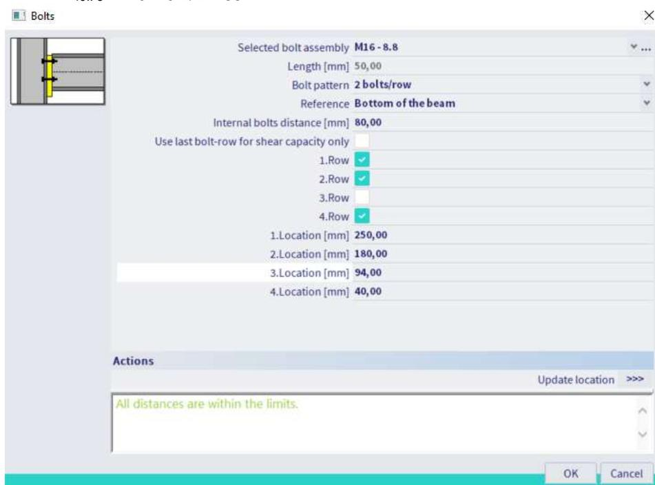
Those values are calculated as the distance from the bolt to the middle of the bottom flange. In SCIA Engineer the values are given as the distance to the bottom of the beam, so we have to subtract the half of the thickness of the flange ( $=9,2 \text{ mm} / 2$ ) of this distance.
