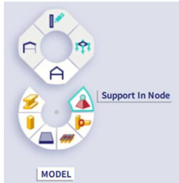
We will add the supports for the **base jacks** (at the bottom nodes of the lowest standards) as nonlinear supports. In the vertical direction these supports can only take pressure and no tension. This is entered in the Z direction with **rigid press only**. The rotations are taken free in all directions.
