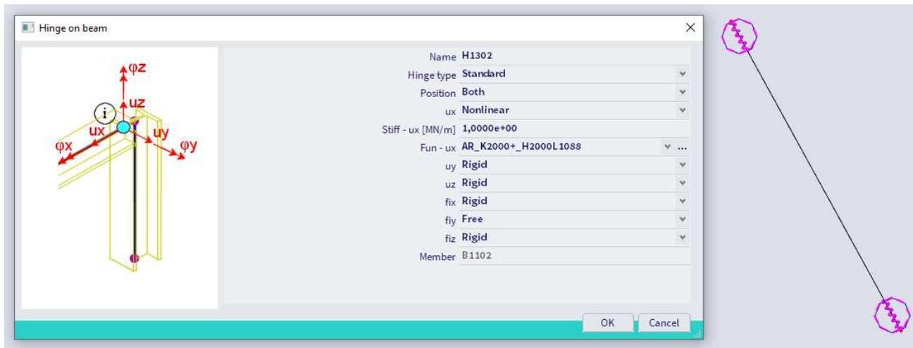
Alternatively diagonals could be modelled via Nonlinearity 1D (**Input panel > Workstation Structure > Category Boundary conditions > Nonlinearity 1D**). Possibilities are:
