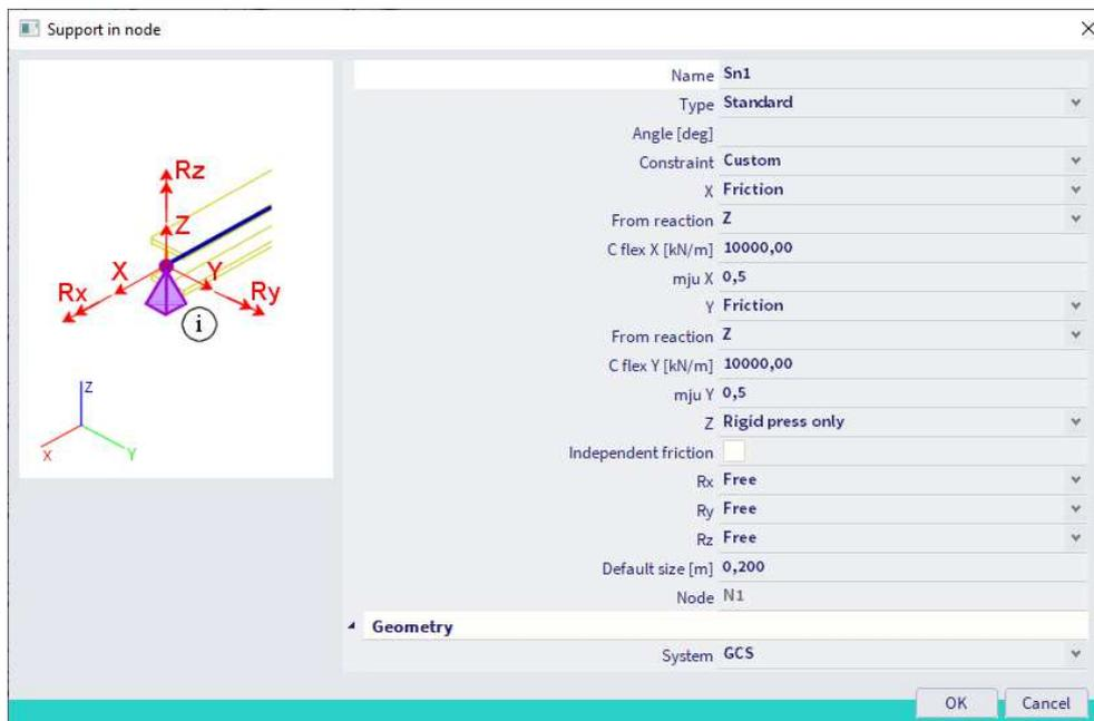
**Note:** independent friction is turned off since this corresponds to a single support that could slide in two directions. For instance, the foot of a scaffolding support. There would be friction behaviour defined in X and Y directions, linked to the vertical reaction. The vertical reaction contributes to both horizontal directions together.
