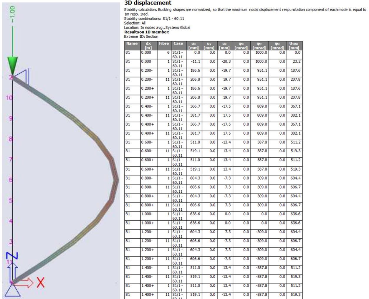
Using for example an Excel worksheet, the buckling shape can be approximated by a 4<sup>th</sup> grade polynomial.
