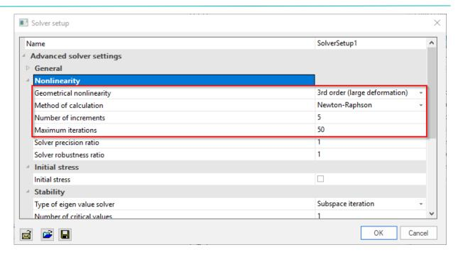
Since the non-linear stability calculation automatically implies the Modified Newton-Raphson method for the solver, this method cannot be chosen here. The reason why this field is available is to perform a normal 3<sup>rd</sup> Order Calculation using Modified Newton-Raphson instead of a Stability Calculation.
