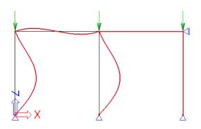
The loading F on each column is 100 kN so the critical buckling load  $N_{\text{cr}}$  can be calculated as:
