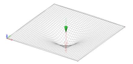
Especially in the corners, tensile contact stresses are expected:
