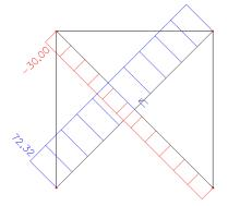
In the left frame, the diagonal has buckled so the tensile force in the remaining diagonal is augmented. In the right frame, the diagonal stays in the structure but yields plastically and thus acts at the limit force of -30 kN.
