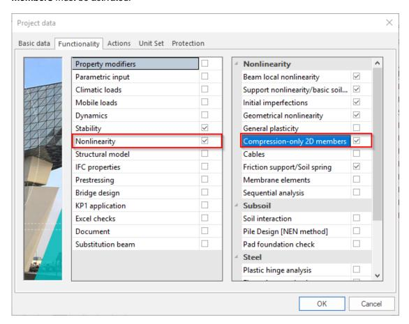
With this option, tension in 2D elements can be automatically eliminated. This is mostly used for masonry elements. In below some examples are shown to clarify this option.
