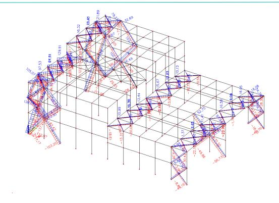
The normal forces for the **non-linear analysis** shows that diagonals are now only subjected to tension thus buckling will not occur anymore. Only very small compression forces will appear in the diagonals.
