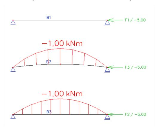
As expected, the beam B1 does not produce a bending moment. Both the curved beam and the beam with imperfection yield the 1 kNm.
