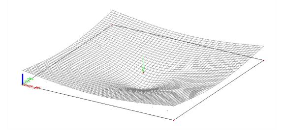
As can be seen, the slab will rise at the corners so no more tensile contact stresses are obtained:
