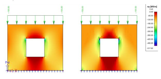
In these results the real pressure of this element is visible for the right element. Looking at the trajectories of this normal force, the trajectory of the pressure force will be even more visible:
