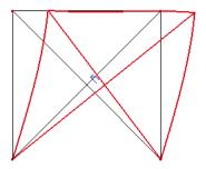
Due to the fact one diagonal has buckled in the left frame, larger horizontal deformations occur.
