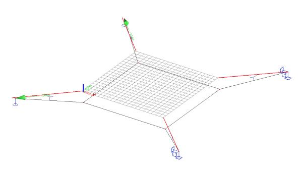
When the scale of the results is augmented, the typical deformation of the membrane element can clearly be seen:
