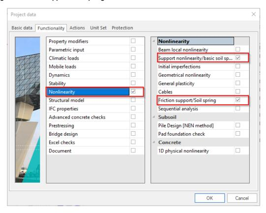
When entering a nodal support, the option **Friction** can be chosen for the translational degrees of freedom (**X**, **Y**, **Z**).
