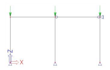
To obtain precise results, the number of 1D elements is refined through **Calculation, mesh > Mesh setup**.
