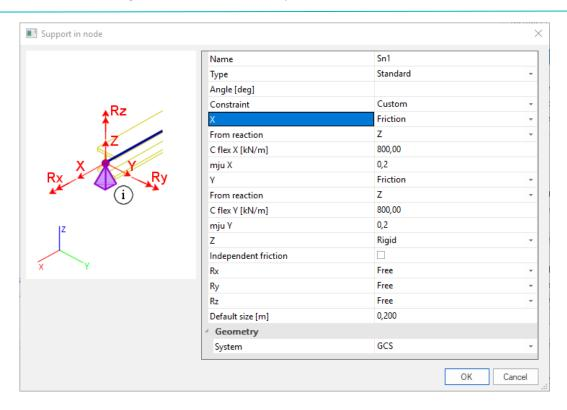
The option From Reaction is used to specify which force component causes the friction force.
