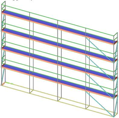
The base jacks are inputted as friction supports. Since a base jack, by default, is not connected to the surface, the Z-direction is defined as rigid **Pressure-only**. Both horizontal degrees of freedom X and Y are defined as **Friction**, dependent on the reaction Z.
