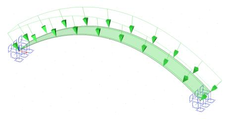
Using an Average Mesh size of 2D element of 0,1m, a Stability Calculation yields the following critical load factor:
