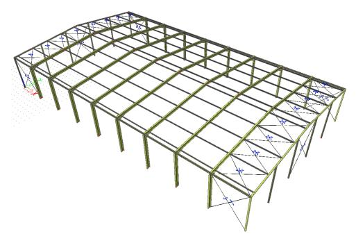
The diagonals have been inputted as **Tension only** members. **Inclination functions** are defined **According to the code** so the initial sway is calculated automatically:
