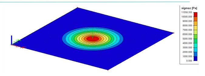
The pressure stresses in the middle have increased which is expected when the slab can rise at the corners.
