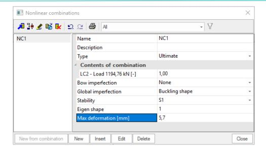
Using this combination, a non-linear 2<sup>nd</sup> Order calculation is executed using Timoshenko's method.
