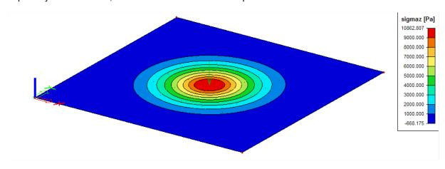
A **non-linear analysis**, taking into account the pressure-only characteristic of the subsoil shows the following deformation:
