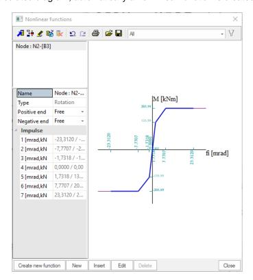
The function characterizes both tension-on-top and tension-at-bottom.
