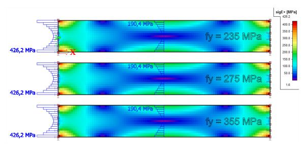
As expected, the Von Mises stresses for every wall are exactly the same and are higher than the yield strength fy.
