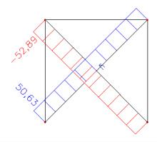
A **non-linear analysis**, taking into account the limit force gives the following results for the normal forces:
