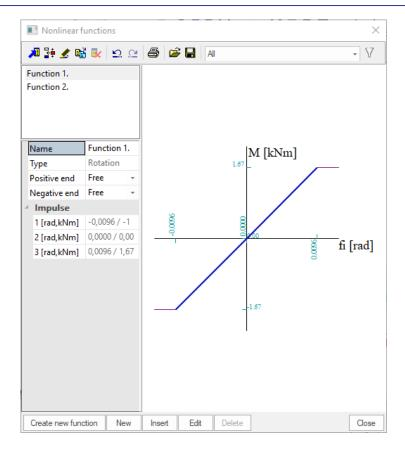
The beam-to-column connections are defined by the following non-linear characteristic:
