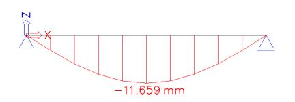
Due to the fact that the self weight causes this deformation, the compression force of 20 kN will lead to an additional moment.
