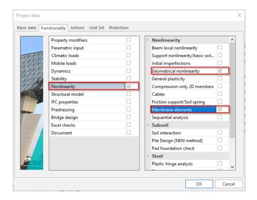
When defining the 2D element, the option **Membrane** must be chosen as FEM nonlinear model.
