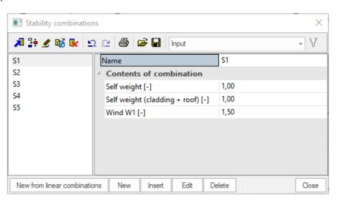
As specified for the non-linear combinations, it is possible to import the linear combinations as stability combinations.
