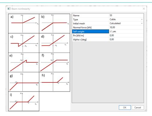
The initial shape will be in equilibrium in relation to the specified load on the cable: either the **Self-weight** or a distributed load **Pn**.
