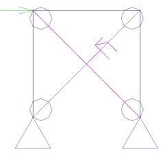
A **linear analysis** shows the following normal forces in the diagonals of both frames:
