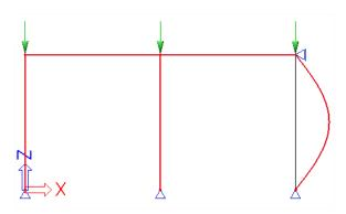
Buckling mode 2 – Critical load factor  $\lambda = 2,89$
