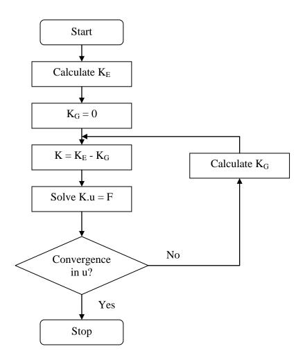
In this figure, the stiffness K is divided in the elastic stiffness  $K_E$  and the geometrical stiffness  $K_G$ . The geometrical stiffness reflects the effect of axial forces in beams and slabs. The symbol u depicts the displacements and F is the force matrix.
