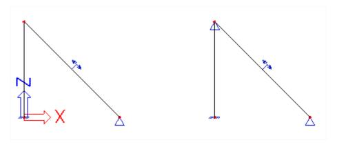
In the left frame, the Initial Stress will immediately be distributed to the column. In the right frame, the extra support will prohibit this.
