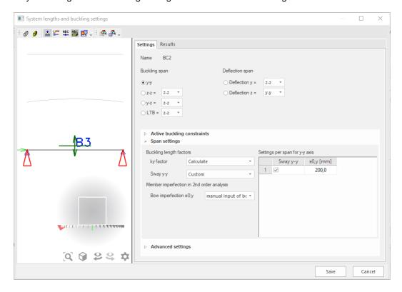
The three beams are loaded by a normal force of **5 kN**. Those with a deflection of 200 mm, are expected to have a moment of **1 kNm** in the middle of the beam.
