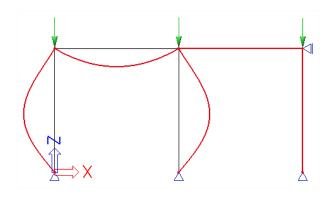
Buckling mode 3 – Critical load factor  $\lambda = 3,53$
