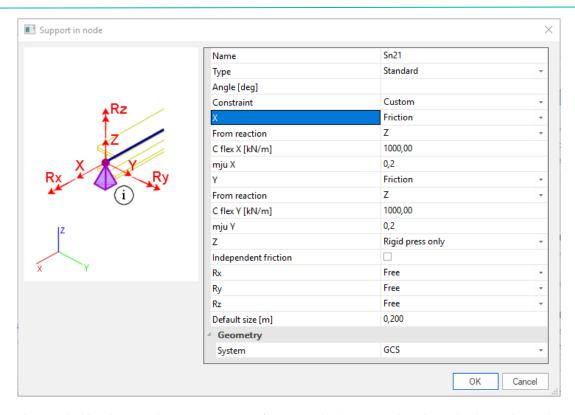
When large wind loads are taken into account, for example due to netting, large horizontal reaction forces are expected in the base jacks. When these reactions surpass the friction force, the support slips through.
