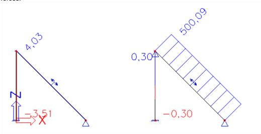
As specified, in the left frame, the initial stress is immediately distributed to the rest of the structure so the tensile force of 500 kN is not found entirely in the diagonal. In the right frame, the force cannot be distributed due to the support so the 500 kN stays in the diagonal.
