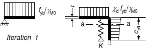
d) Reduced strength  $\chi_d f_{yb} / \gamma_{M0}$  for effective area of stiffener  $A_s$ , with reduction factor  $\chi_d$  based on  $\sigma_{cr,s}$
