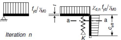
e) Step 3: Optionally repeat step 1 by calculating the effective width with a reduced compressive stress  $\sigma_{com,Ed,i} = \chi_d f_{yb} / \gamma_{M0}$  with  $\chi_d$  from previous iteration, continuing until  $\chi_{d,n} \approx \chi_{d,(n-1)}$  but  $\chi_{d,n} \leq \chi_{d,(n-1)}$ .
