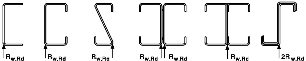
**Figure 6.6: Examples of cross-sections with a single web**
