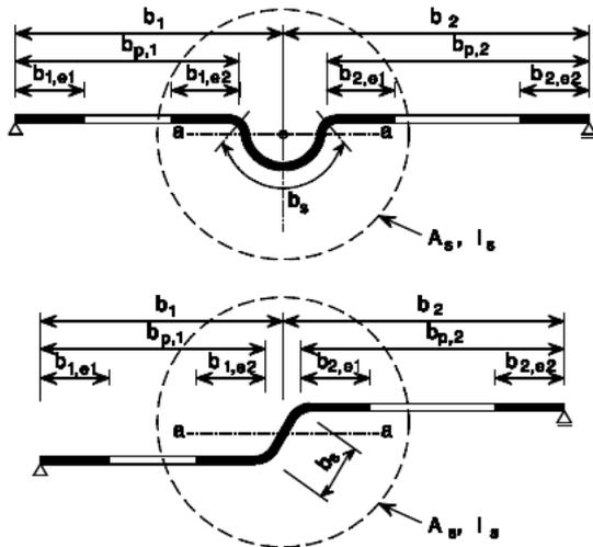
Figure 5.9: Intermediate stiffeners
