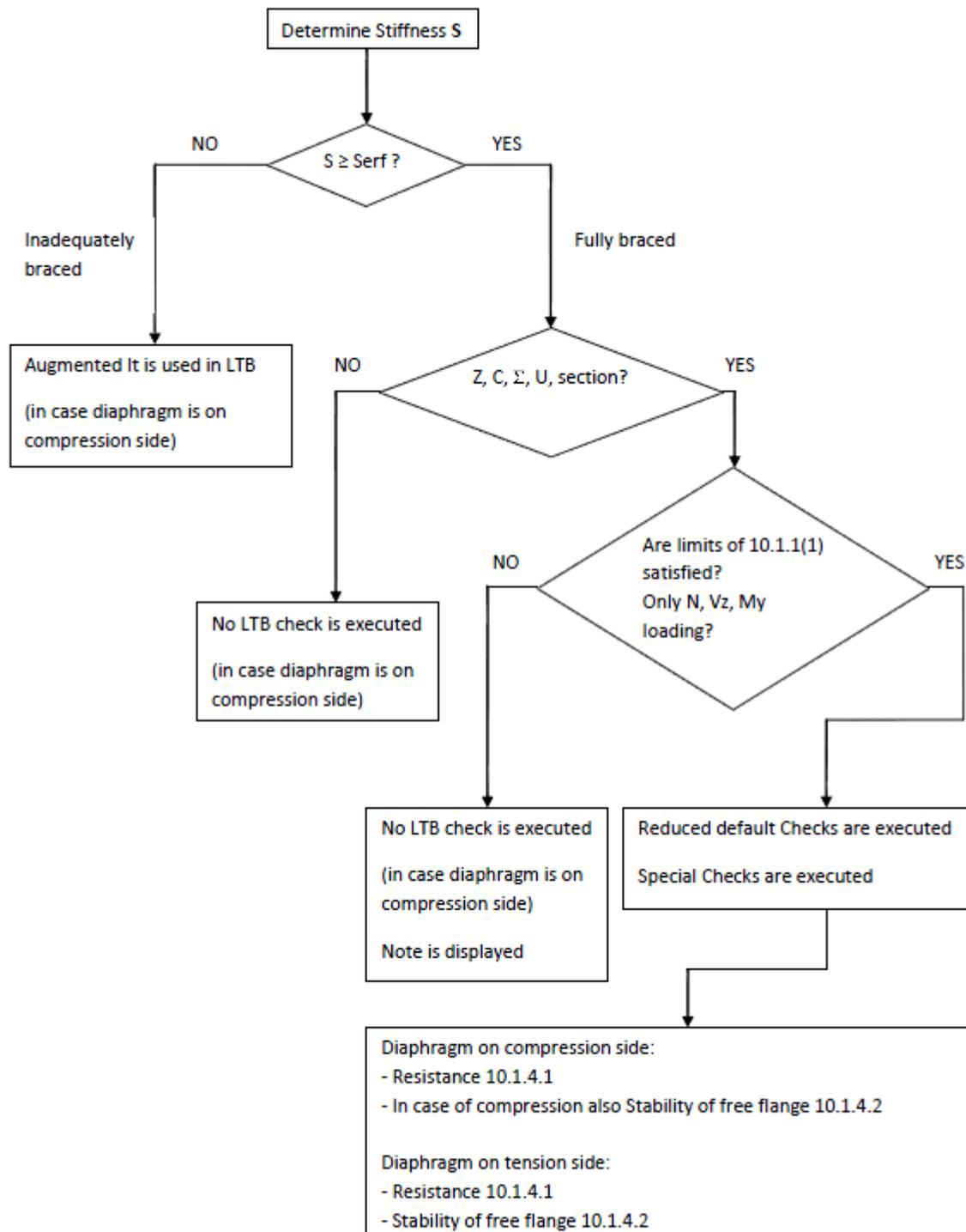
$$S = \frac{a \cdot 10^4}{K_1 + \frac{K_2}{L_s}} S_{erf} = \left( E I_w \frac{\pi^2}{L^2} + G I_t + E I_z \frac{\pi^2}{L^2} 0,25 h^2 \right) \frac{70}{h^2} I_{t,id} = I_t + vorC_\theta \frac{l^2}{\pi^2 G}$$
