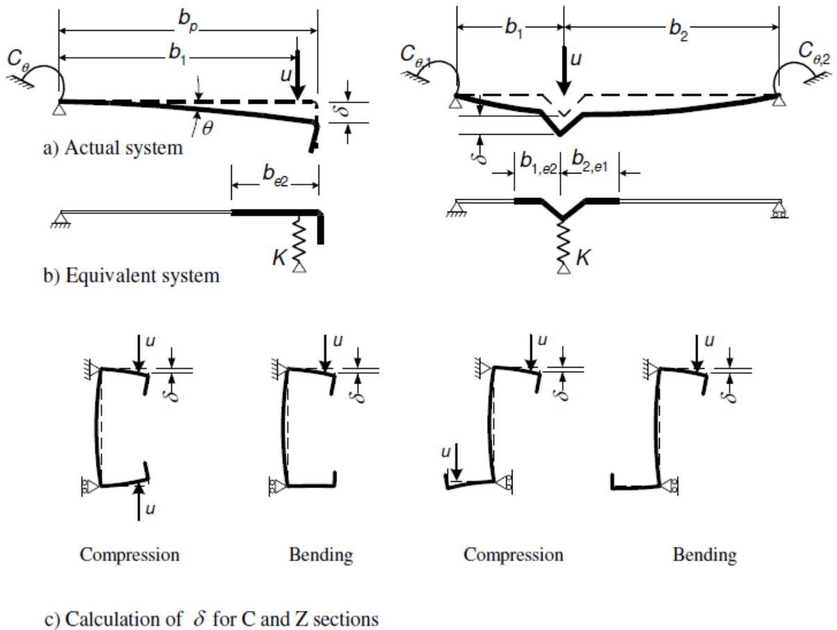
Figure 5.6: Determination of spring stiffness
