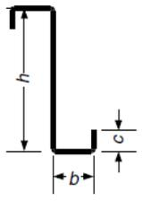
$k_{h0} = \frac{ht(b^2 + 2cb - 2c^2b/h)}{4I_y}$ <p>Simple symmetrical Z section</p> |
