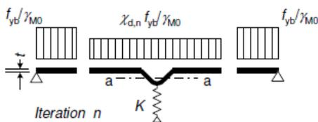
e) Step 3: Optionally repeat step 1 by calculating the effective width with a reduced compressive stress  $\sigma_{com,Ed,i} = \chi_d f_{yb} / \gamma_{M0}$  with  $\chi_d$  from previous iteration, continuing until  $\chi_{d,n} \approx \chi_{d,(n-1)}$  but  $\chi_{d,n} \leq \chi_{d,(n-1)}$ .
