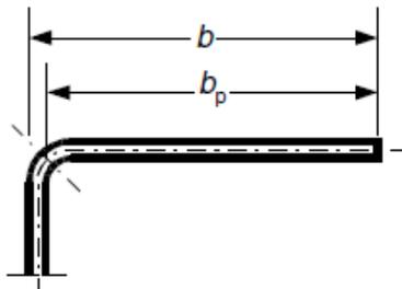
(b) notional flat width  $b_p$  of plane parts of flanges
