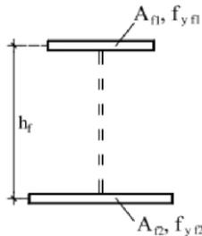
$$M_{f,Ed} = \min \left( h_f \cdot A_{f1} \frac{f_{y,f1}}{\gamma_{M0}}, h_f \cdot A_{f2} \frac{f_{y,f2}}{\gamma_{M0}} \right)$$
