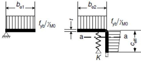
b) Step 1: Effective cross-section for  $K = \infty$  based on  $\sigma_{com,Ed} = f_{yb} / \gamma_{M0}$
