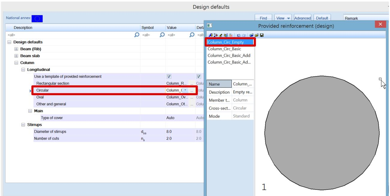
**Remark 2:** According to *EN1992-1-1 art 9.5.2(4)*, there is a minimum number of bars in a circular column. This parameter is set by default to “4” in Concrete Setup > Detailing provisions > Column > Longitudinal.
