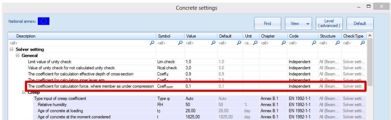
This option 'The coefficient for calculation force, where member as under compression' will check how important the contribution of the axial compression force is:
