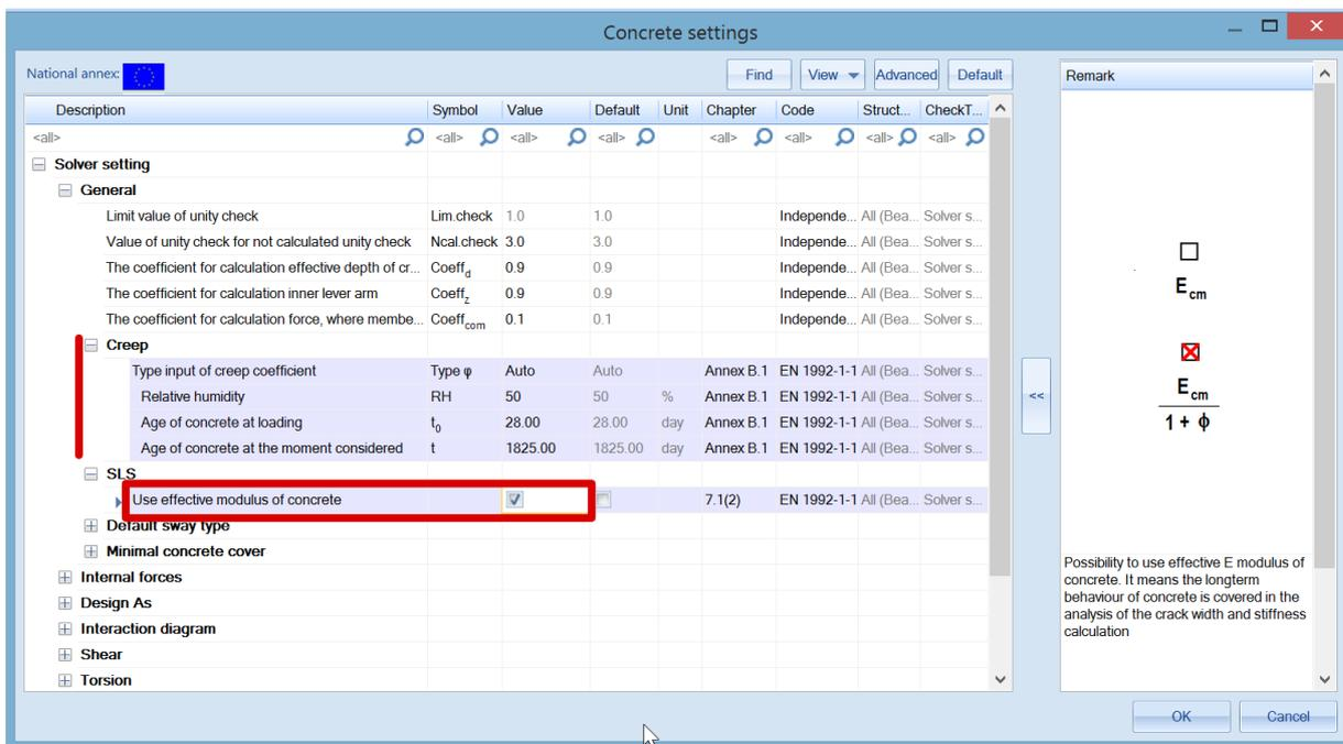
**Note:** Scia Engineer is not able to use characteristic or quasi-permanent combinations together in one step. Therefore, the same forces (load combination) are used for crack appearance and final stress values.
