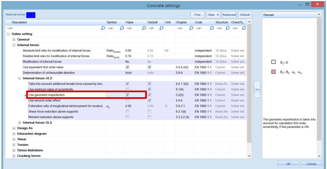
In SCIA Engineer, the geometrical imperfection is represented by an inclination according to clause 5.2(5) in EN 1992-1-1.
