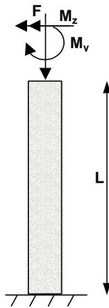
This method allows to design reinforcement for a normal force ( $N_{Ed}$ ) and biaxial bending moments. This method is based on an interaction formula, equation 5.39 in EN 1992-1-1.
