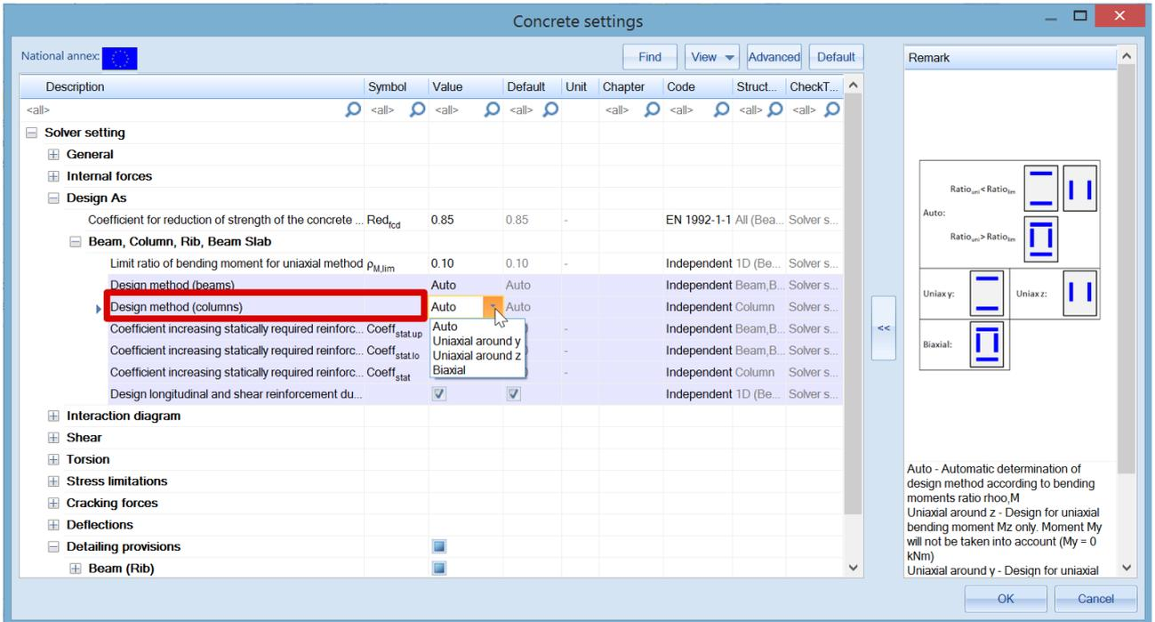
The “Auto” selection of the design method is based on the limit ratio of bending moment for the uniaxial method. The program will automatically select the uniaxial or biaxial method depending on the values of bending moments around y and z axis.
