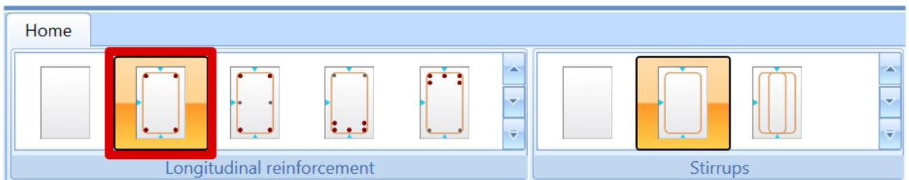
Then change the diameter of the reinforcement template. For bottom longitudinal bars, change diameter to 20mm in the tab "Reinforcement (layout)":
