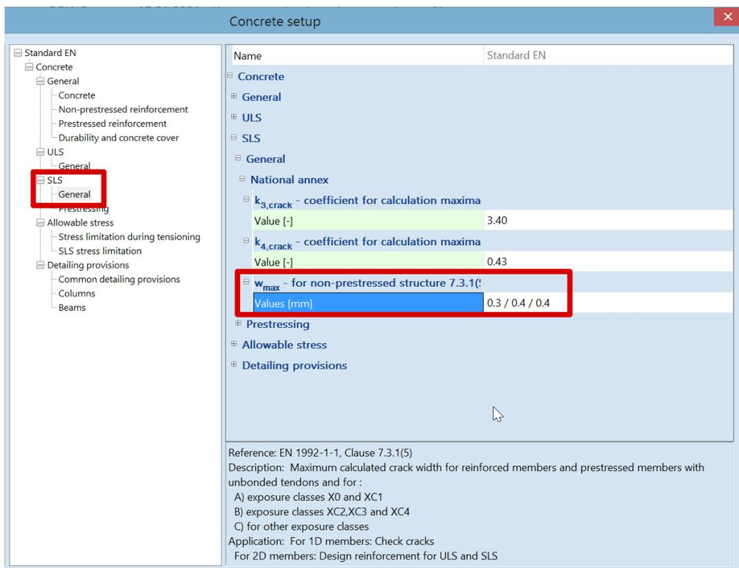
The user can manually input the limiting crack width in Settings per member > 1D member data:
