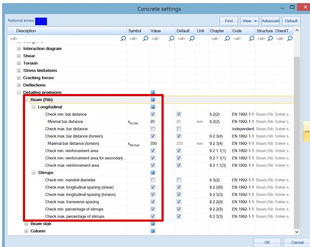
Following table shows which checks of detailing provisions are performed:
