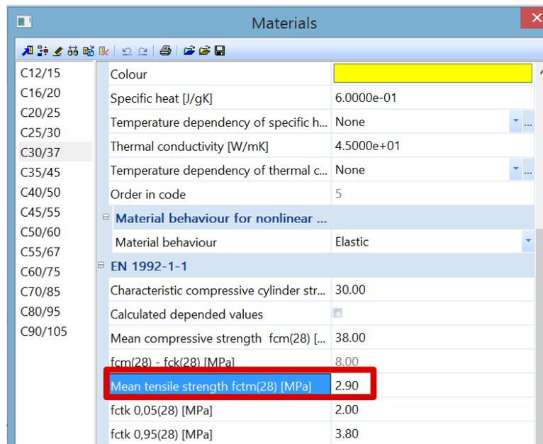
**Note:** The value presented in material properties (picture above) is the mean tensile strength at 28 days. If cracking is expected earlier than 28 days, it is necessary to input this value  $f_{ctm}(t)$  into the material properties (EN 1992-1-1, clause 3.1.2(9)).
