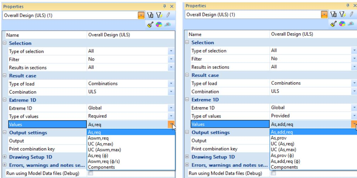
The provided reinforcement  $A_{s,prov}$  gives the amount of reinforcement or in bars ( $A_{s,prov}$ ), determined by the template.  $A_{s,add,req} = A_{s,req} - A_{s,prov}$ , thus the amount of reinforcement which still has to be added to the template to resist the (recalculated) internal forces. If  $A_{s,prov} > A_{s,req}$ ,  $A_{s,add,req} = 0$ . Also unity checks can be performed on the provided reinforcement.
