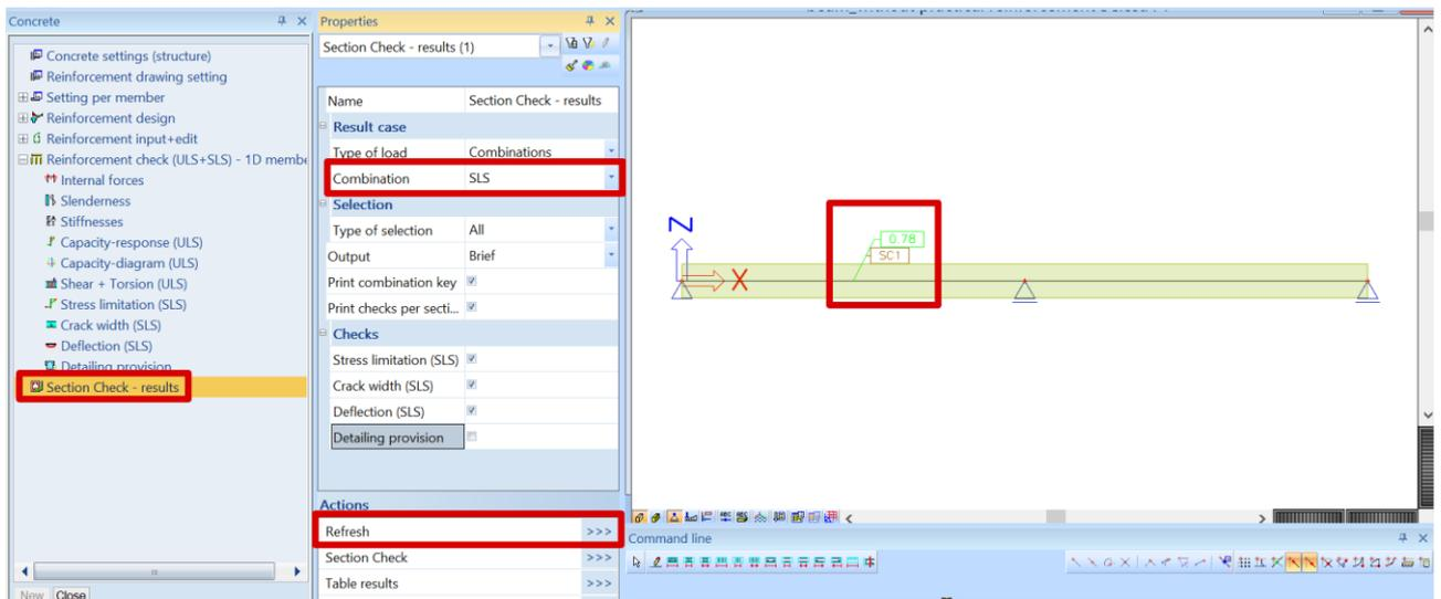
If required, Section check tool can still be opened to redesign the section to satisfy the SLS checks by clicking on Section check in the Properties window.
