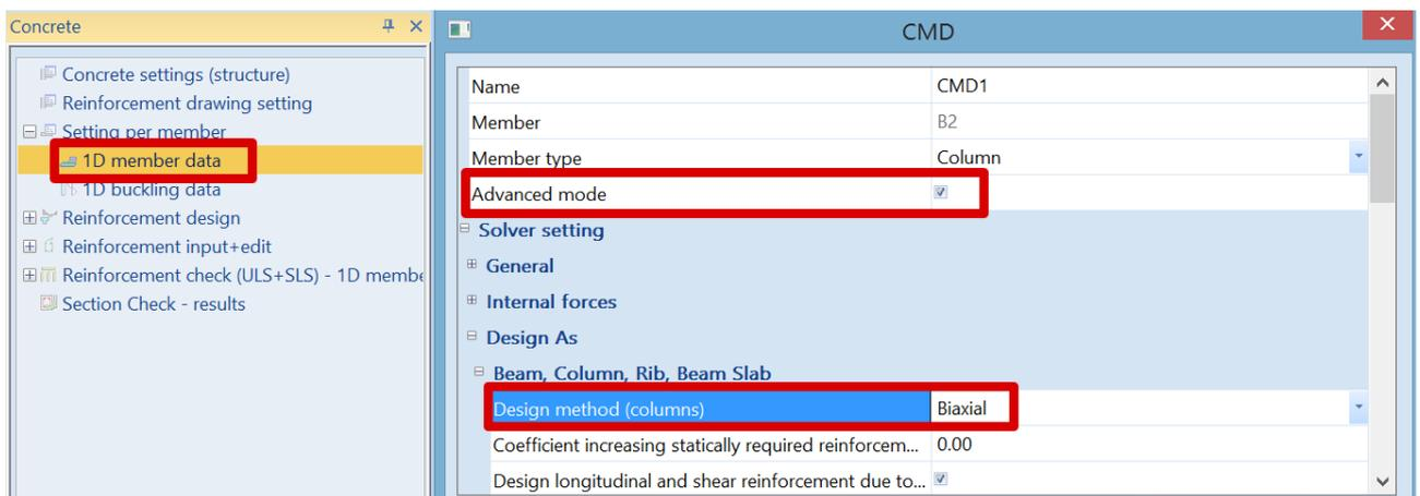
Amount of required reinforcement will be slightly higher in this case since  $M_{Edz}$  is also considered.
