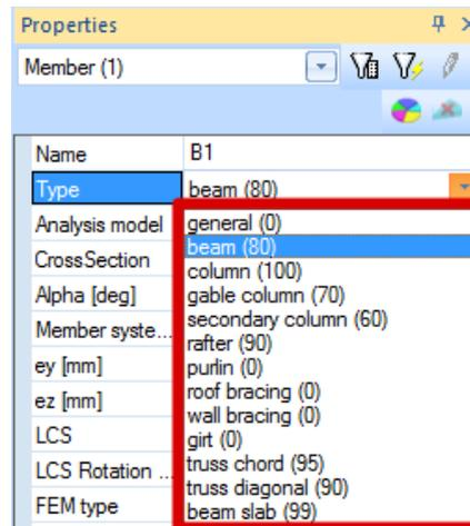
The Beam calculation is used for the Types 'General', 'Beam', 'Rafter', 'Purlin', 'Roof bracing', 'Wall bracing', 'Girt', 'Truss chord' and 'Truss diagonal'.
