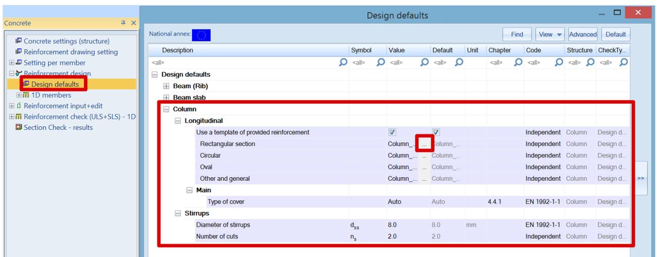
By default, the diameter for the main column reinforcement is put to  $\phi 16\text{mm}$ . Based on this diameter and the exposure class (by default XC3), the concrete cover is calculated. This information is necessary to be able to calculate the lever arm of the reinforcement bars.
