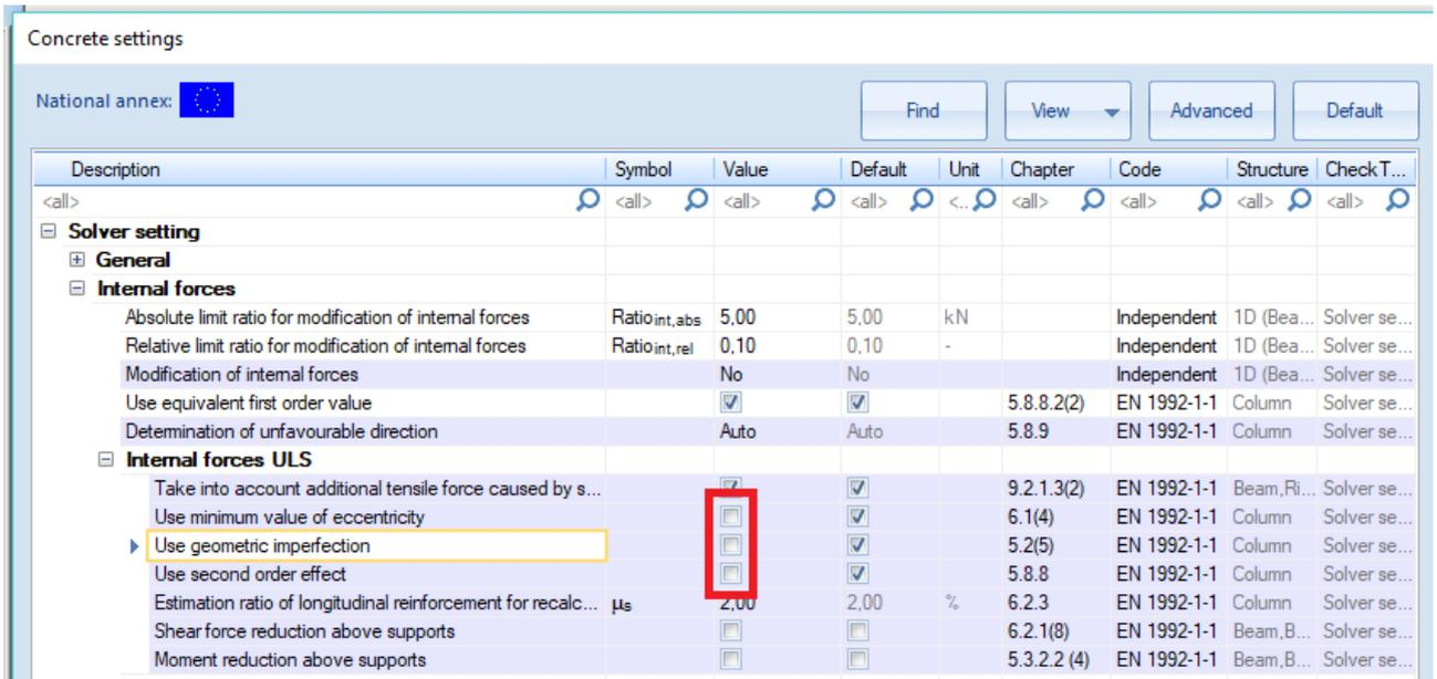
Item Detailing provisions are not taken in account, to view the pure results (according to the Eurocode, always a minimum reinforcement percentage must be added).
