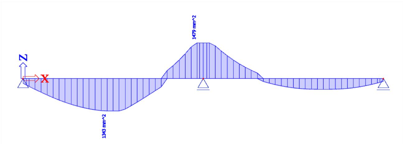
**Longitudinal required reinforcement**
