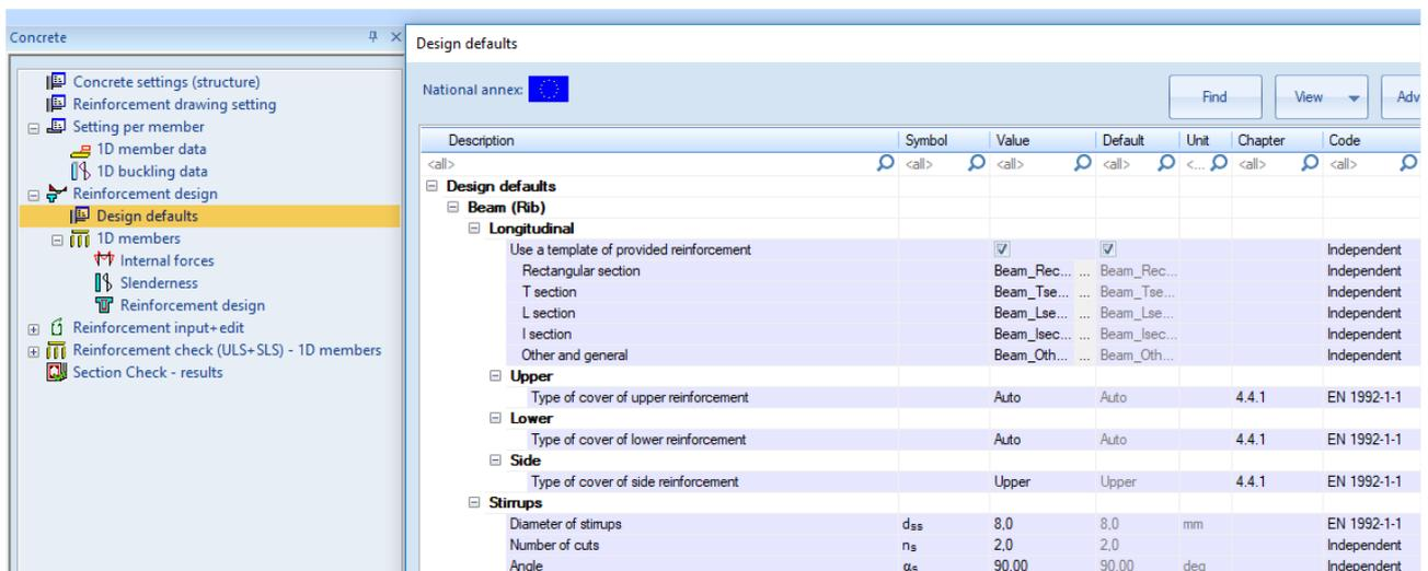
Several default templates for longitudinal reinforcement are available for the different section types. These can be adapted or new ones can be made.
