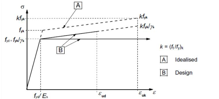
Figure 3.8: Idealised and design stress-strain diagrams for reinforcing steel (for tension and compression)
