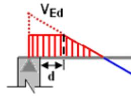
Also for the reduction of shear forces, the support width  $t$  is taken into account, which is taken from the properties of the support or the 1D member data.
