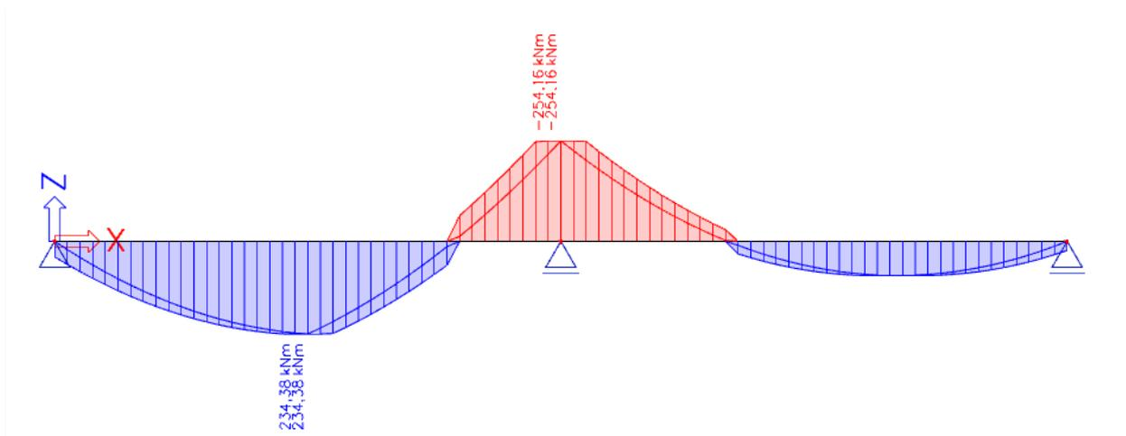
The shifted moment line is taken into account for recalculated internal forces and by this also for the calculation of longitudinal reinforcement, if activated in the concrete settings (for the global structure) or in the 1D member data (individually per member):
