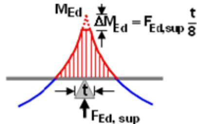
In SCIA Engineer the width  $t$  used for the moment reduction at supports can be set in the properties of that support:
