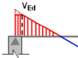
**At the face of the column + effective depth of the cross-section (based on 6.2.1 (8))**
