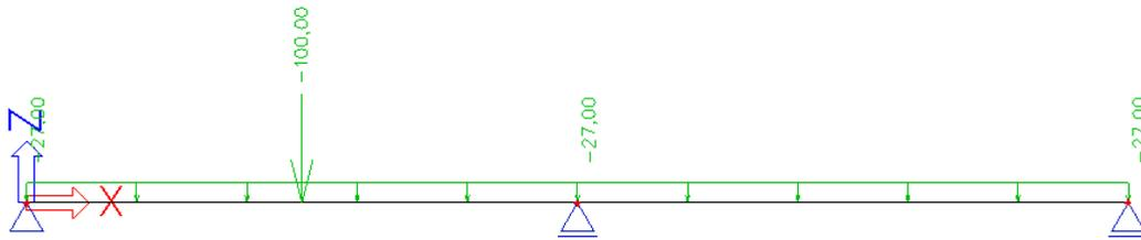
The length of the total beam is 10 m and it has a dimension of 500x300mm.
