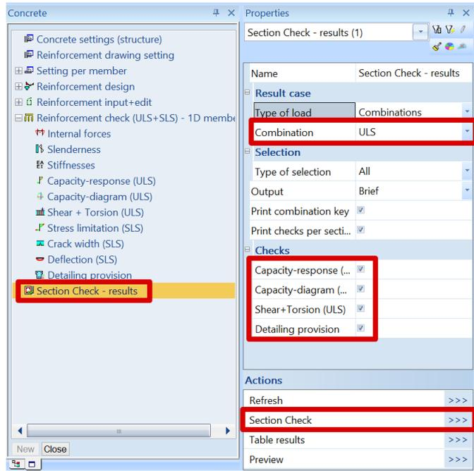
Select Section 9, in the middle of the first span.
