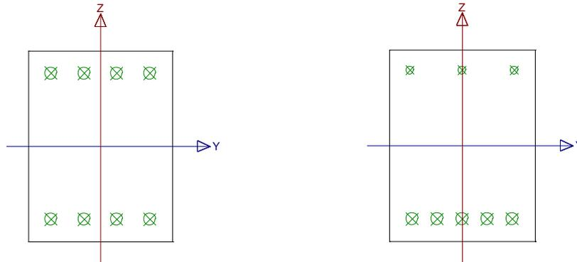
These configurations are obvious, and caused by the difference in dominant internal forces per calculation type. For a beam calculation the bending moment is dominant, while for a column calculation the axial compression force + bending moments (if present).
