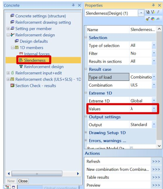
The Standard output shows the check of  $\lambda > \lambda_{lim}$  and indicates whether a 1<sup>st</sup> or 2<sup>nd</sup> order calculation should be done.
