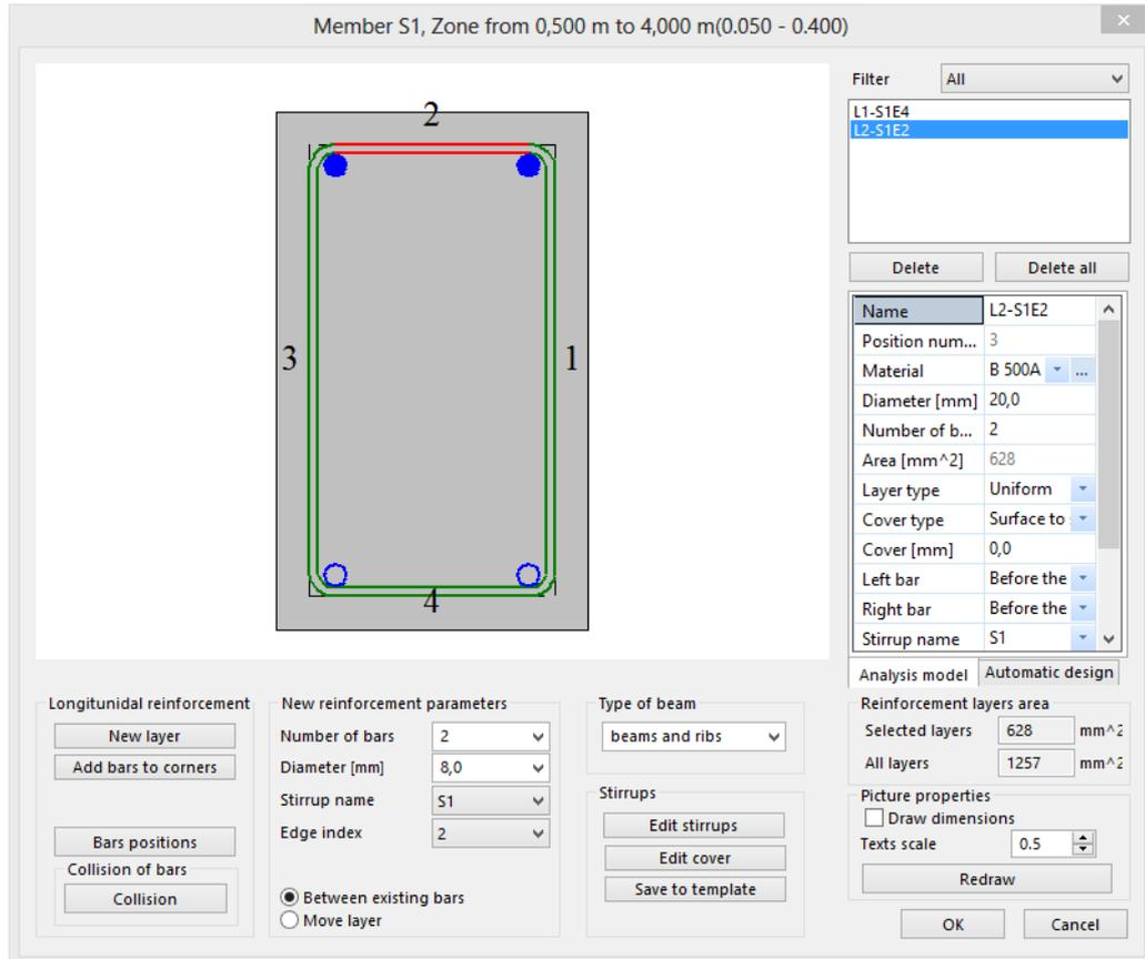
Here can be set on which face extra reinforcement needs to be added:
