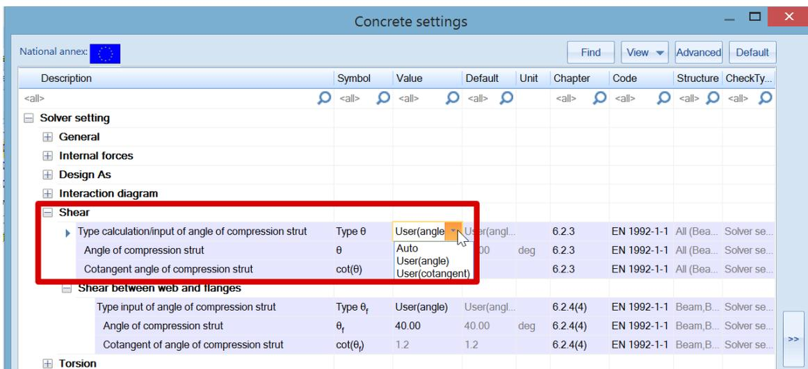
The angle should be between  $\theta_{min}$  and  $\theta_{max}$  defined in the NA for EN1992-1-1.
