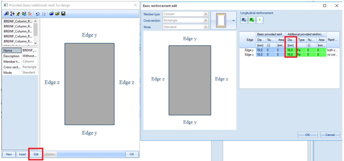
**Note:** To change the default diameter from  $\phi 16\text{mm}$  to  $\phi 20\text{mm}$  for example, edit the template "Column\_Rect\_Empty" (or the corresponding empty template for the specific columns shape), and change the value of the diameter to be taken into account (additional provided reinforcement).
