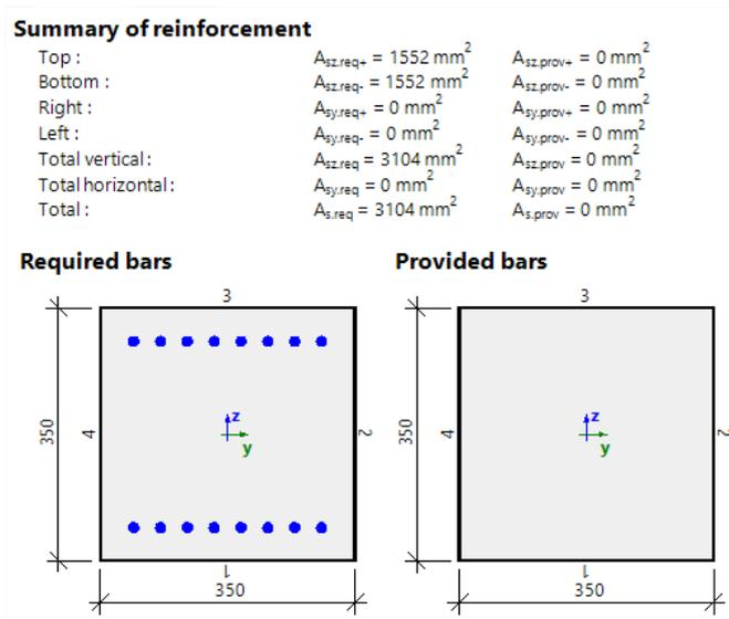
Even if an additional bending moment in the z direction is present in column B2, according to the limit ratio the uniaxial method was used, and the same amount of reinforcement is required for columns B1 and B2.
