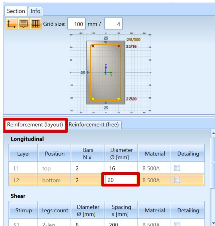
Note that it is also possible to define the shear reinforcement in this window.
