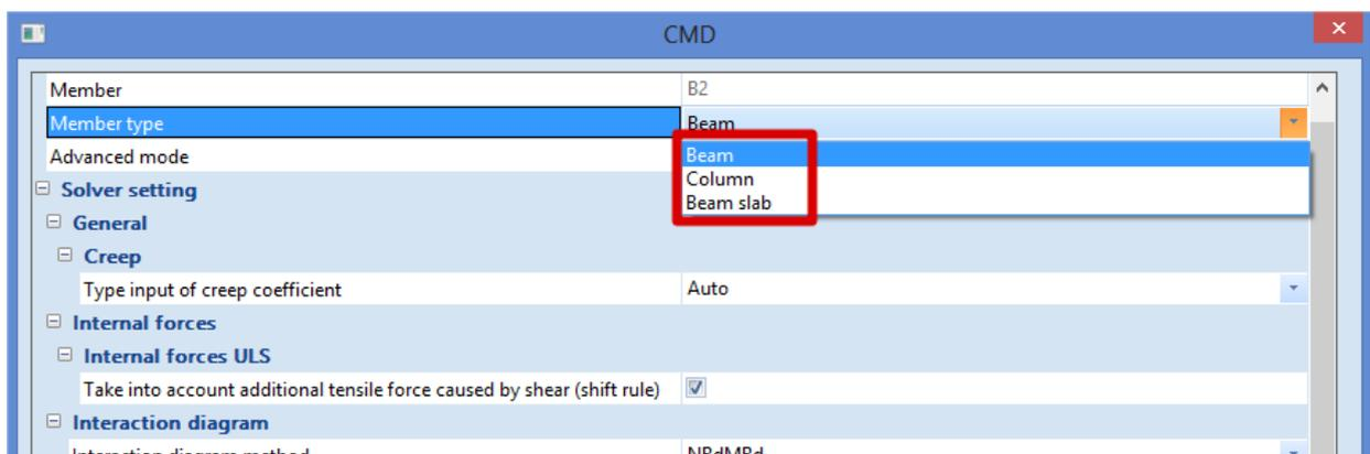
**These 1D member data *overwrite* both the element properties and the default settings in the Concrete settings.**
