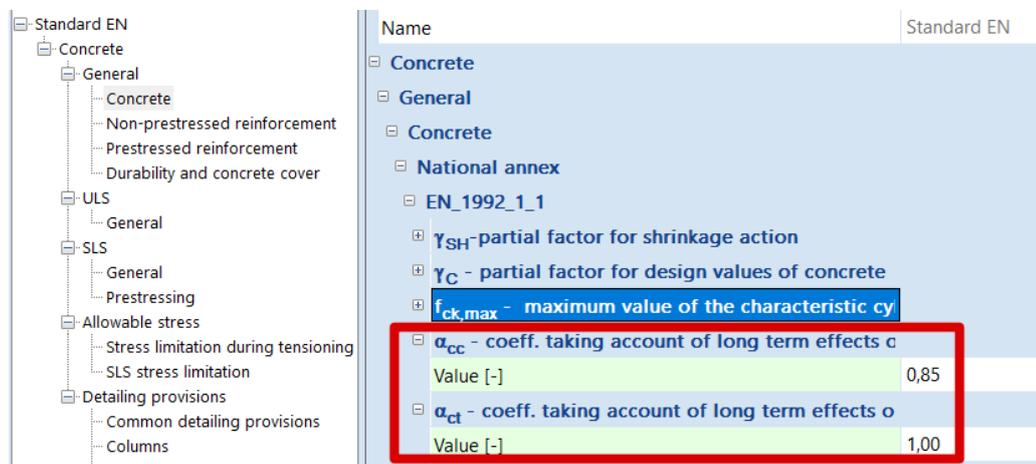
If the concrete strength is determined at an age  $t > 28$  days the values  $\alpha_{cc}$  and  $\alpha_{ct}$  should be reduced by a factor  $k_t$ .
