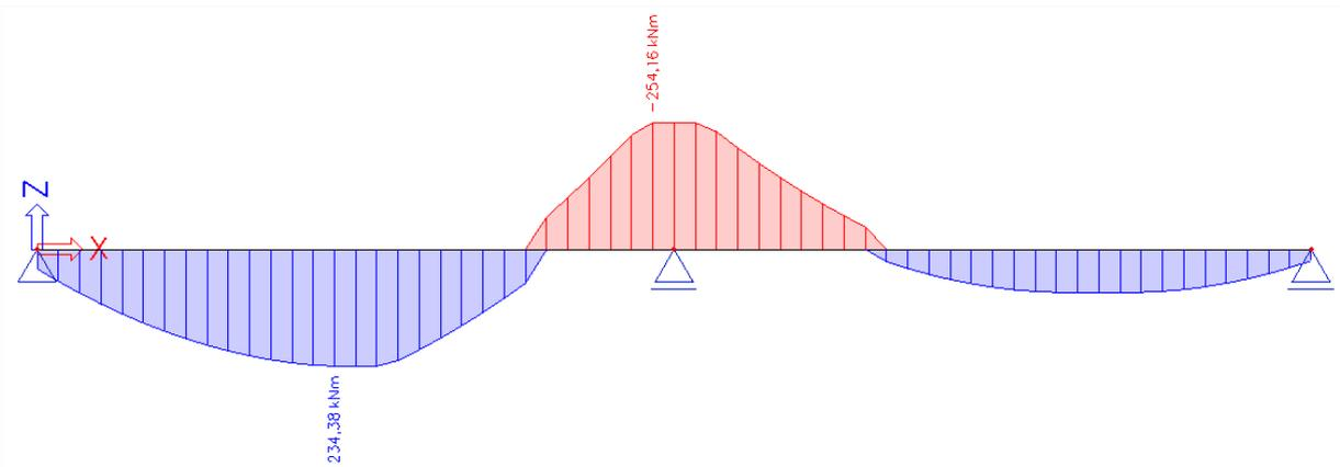
With moment capping at support taken into account the recalculated moment is 242.22 kNm.
