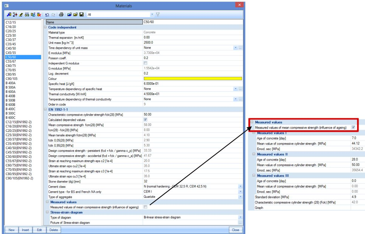
It may be required to specify the concrete compressive strength,  $f_{ck}(t)$ , at time  $t$  for a number of stages (e.g. demoulding, transfer of prestress), where:
