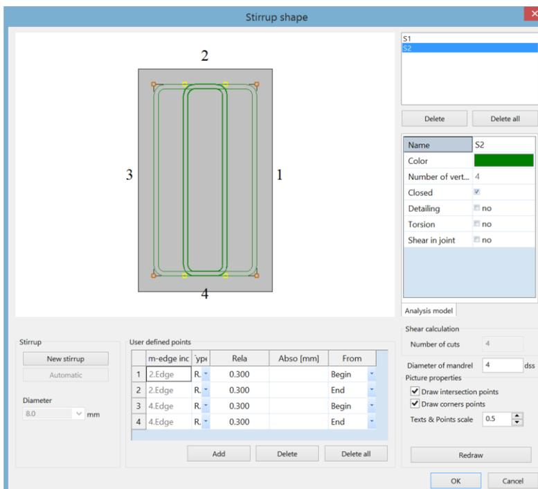
Changing the stirrup shape allows us to keep a bigger distance of 0.2m between stirrups in "Zone 2".
