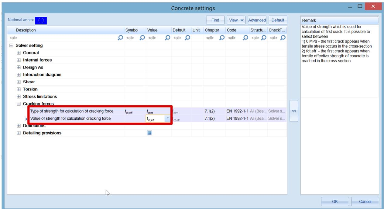
**Value of strength for calculation of cracking forces:**
