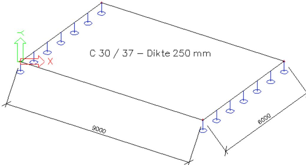
\*Input plate: Structure menu > 2D Member > Plate
