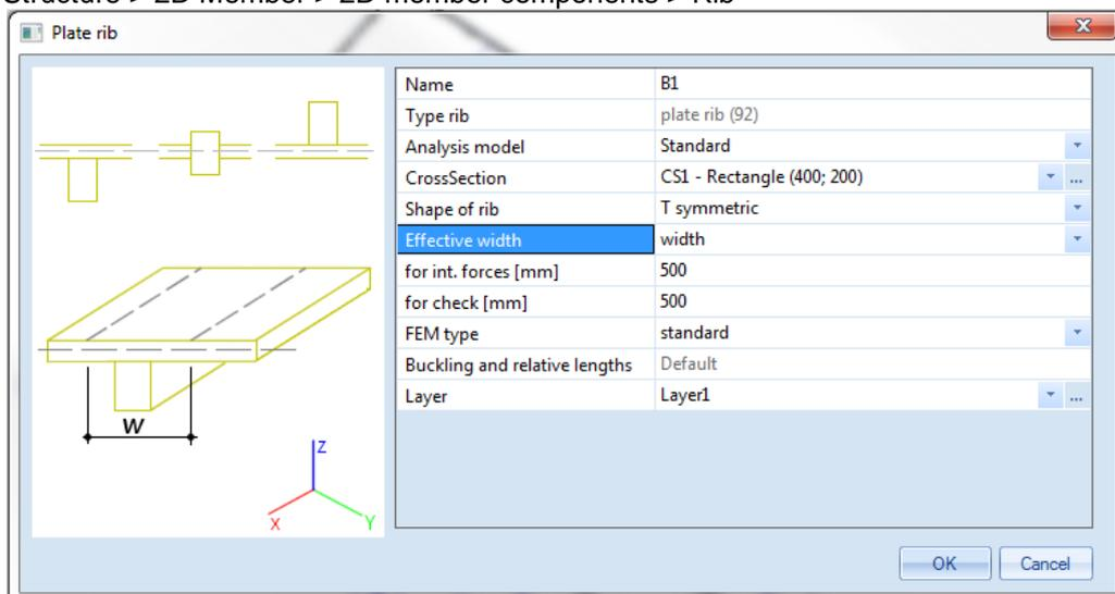
Effective width = Default, Number of plate thickness, or Width in mm
