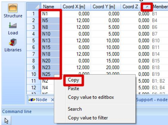
Copy the names of the nodes with a Z=0m and paste it in MS Excel
