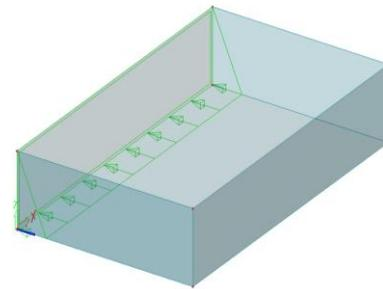
Input the geometry of the free load as a New rectangle in the XY plane
