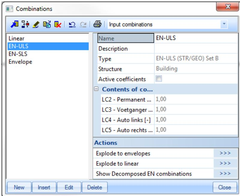
'Black Box': As well for combinations according to the Eurocode as for Envelope combinations, the generated *linear* combinations are not shown.
