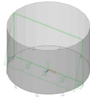
Input the geometry of the free load as a New rectangle in the XY plane
