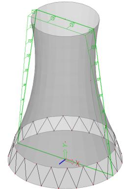
Input the geometry of the free load as a New polygon in the XY plane
