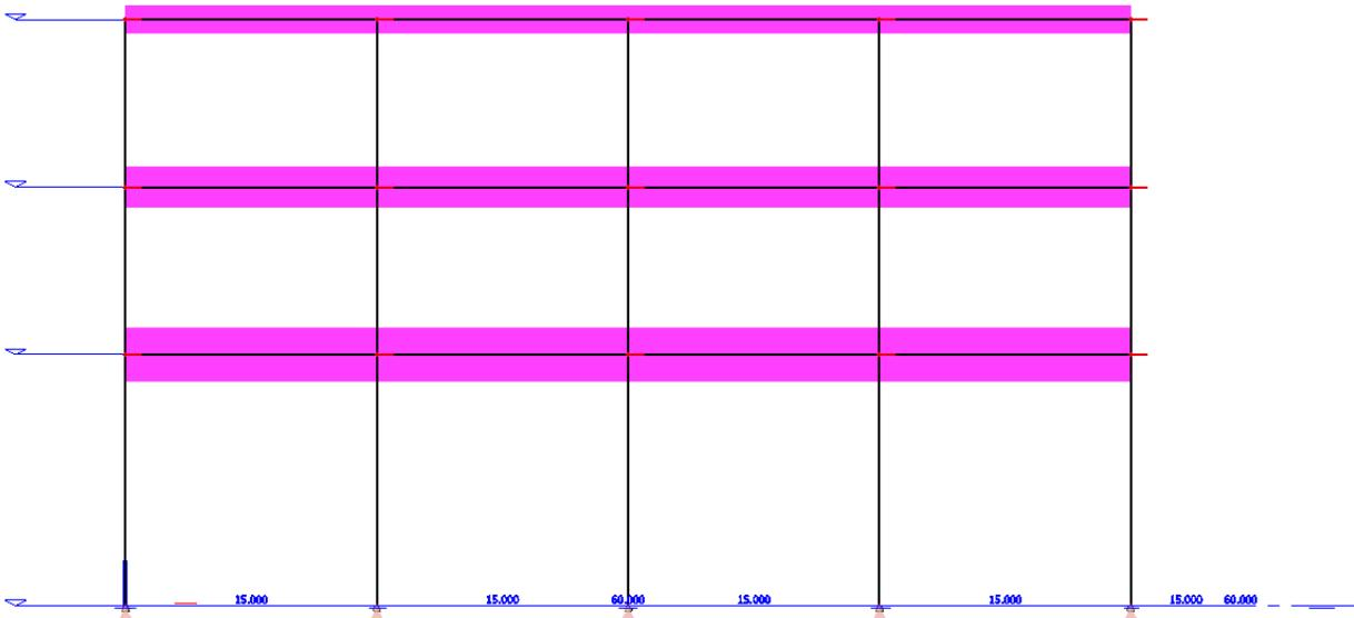
Once the masses are added to the model, a
