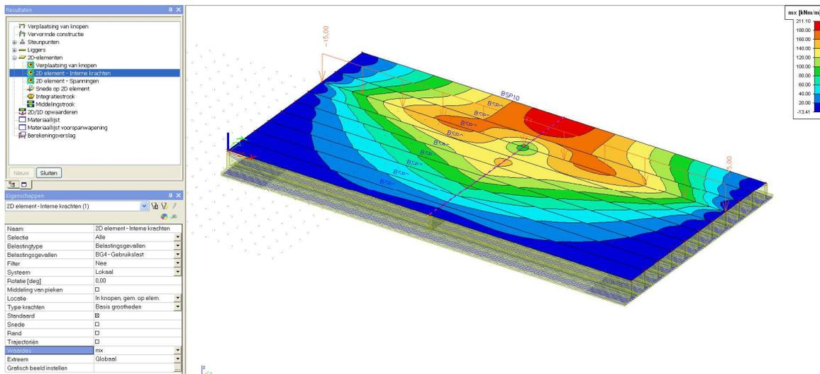
The transverse beam is clearly providing a better spreading of the loads.
