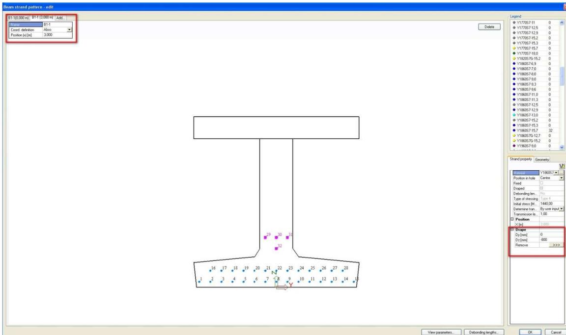
Another measure that could be taken to avoid that in the begin section a tension stress at the top fibre would occur is the debonding of some strands over the first meters. In this example the strands on the bottom row are all given a debonding length of 3m.
