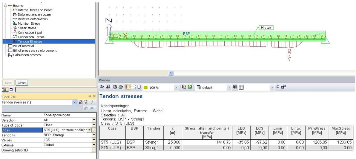
There is clearly an increase in LCS losses between the beginning and the end of the service stage.
