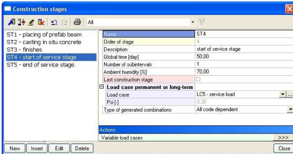
The Psi factor of 0,3 will only influence the participation of LC5 to the long term losses calculated by TDA solver. In the generated combinations, this load case will be considered without this reduction factor, so this reduction factor is only for the calculation of losses, not for the concrete checks.
