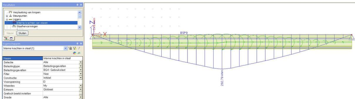
This moment line is a result of integration from the internal forces on the 2D prefab slab model.
