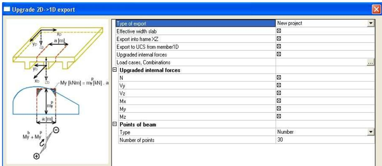
The width of bridge deck that is taken into account in the export is defined by the effective width (which could be entered in the properties of the precast slab). This effective width is also used as integration width to define the equivalent internal forces on the 1D element model.
