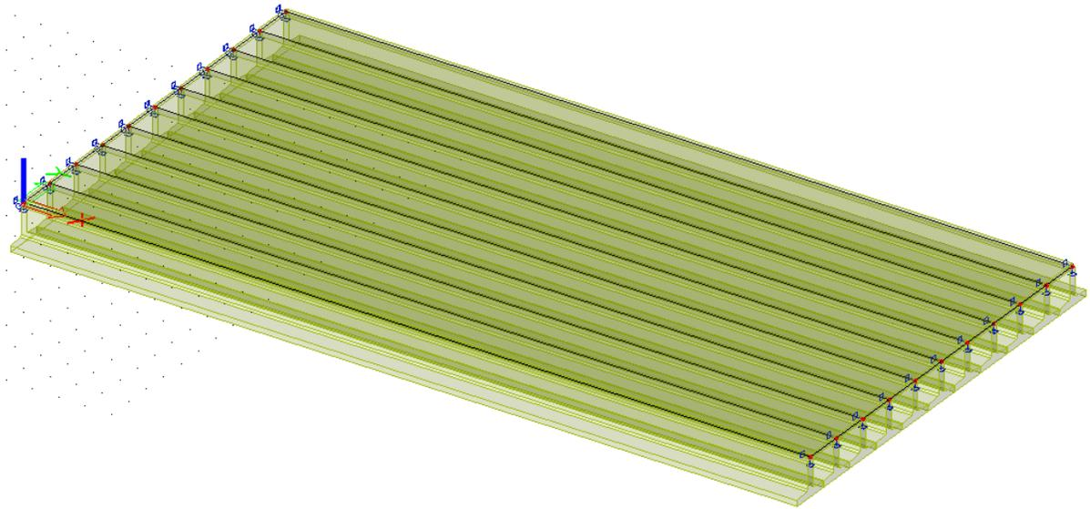
It is also possible to define the prestress reinforcement in this model, but it will not be taken into account for the calculation. It will however be exported to the 1D elementmodel where it will be taken into account in the analysis.
