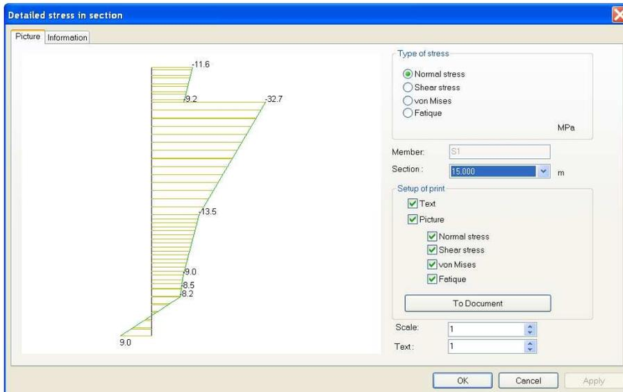
Notice the jump in stress between the two phases of the cross-section.
