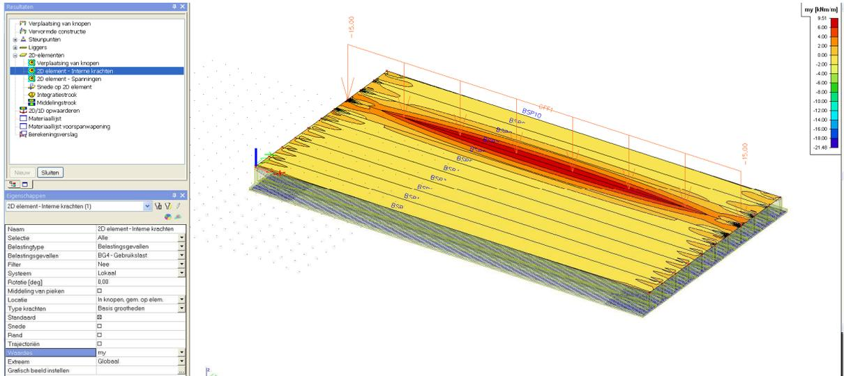
To increase the spreading of the loads, a transverse beam could be added to the model.
