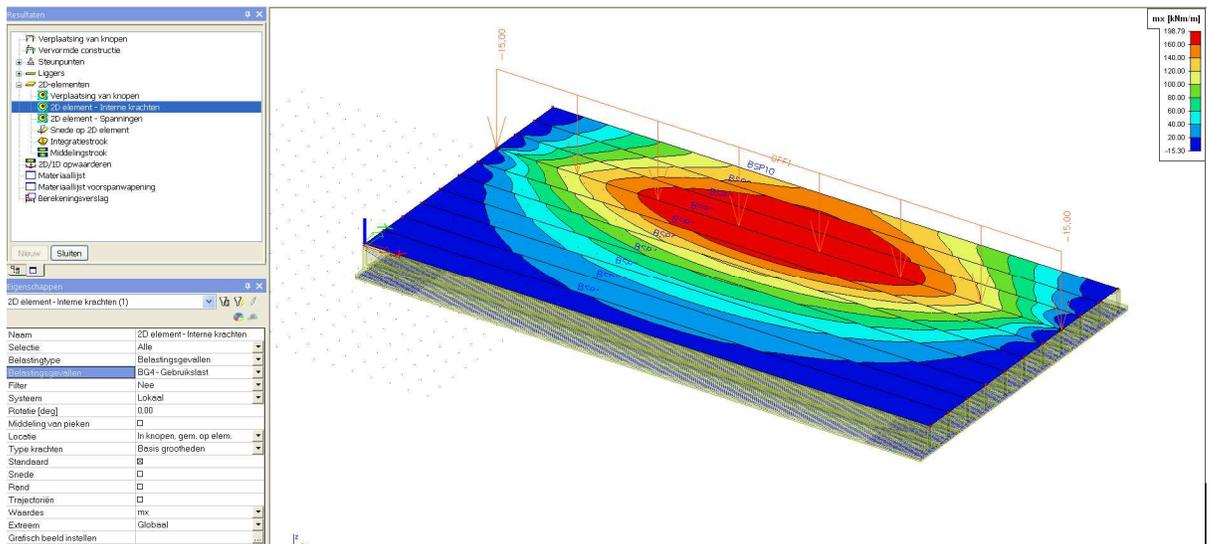
There is a clear spreading noticeable. The local line load of 15kN/m will be spread over multiple beams. This spreading is caused by the transversal stiffness of the prefab plate model. This transversal stiffness will be delivered by the in situ topping of the bridge deck (and not by the prefab beam elements themselves who will serve of course for the longitudinal stiffness).
