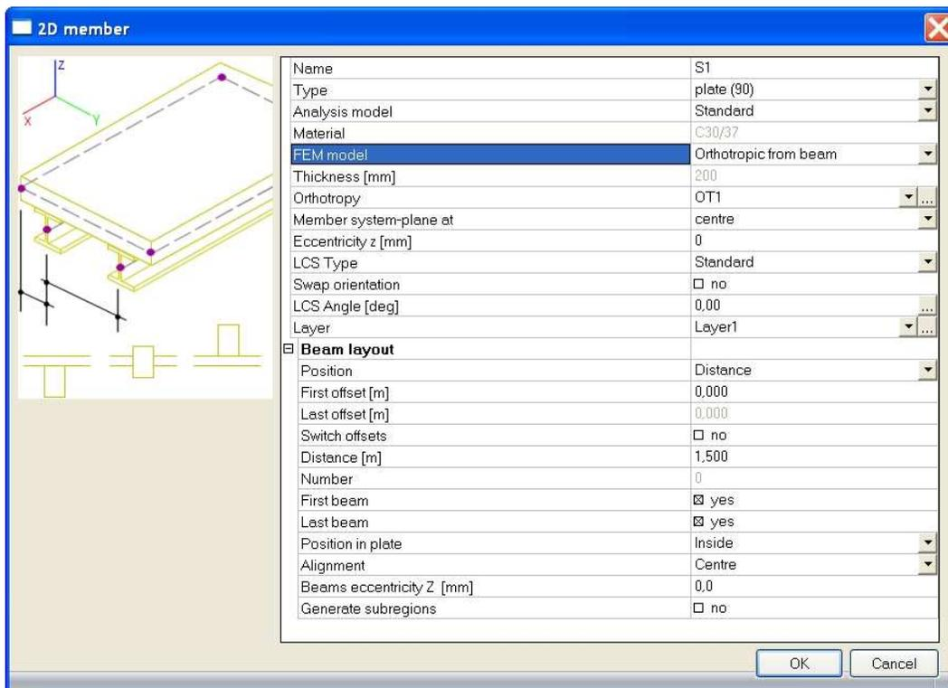
To assign a correct stiffness to the plate, which is of course important for the load distribution, the FEM model of the plate will be set to orthotropic. As type of orthotropy the OT type 'slab with ribs' could be used. The stiffness will then be calculated based upon the orthotropic parameters. Only the self weight is not yet taken into account correctly then, but this is no problem, since it can be recalculated in the 1D element model.
