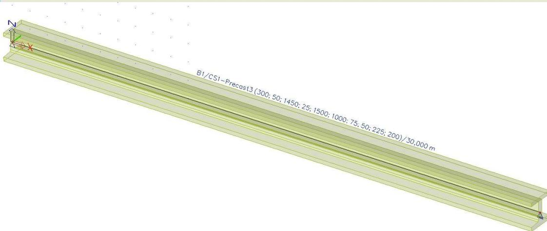
The input of the pretensioning is done in the concrete menu.
