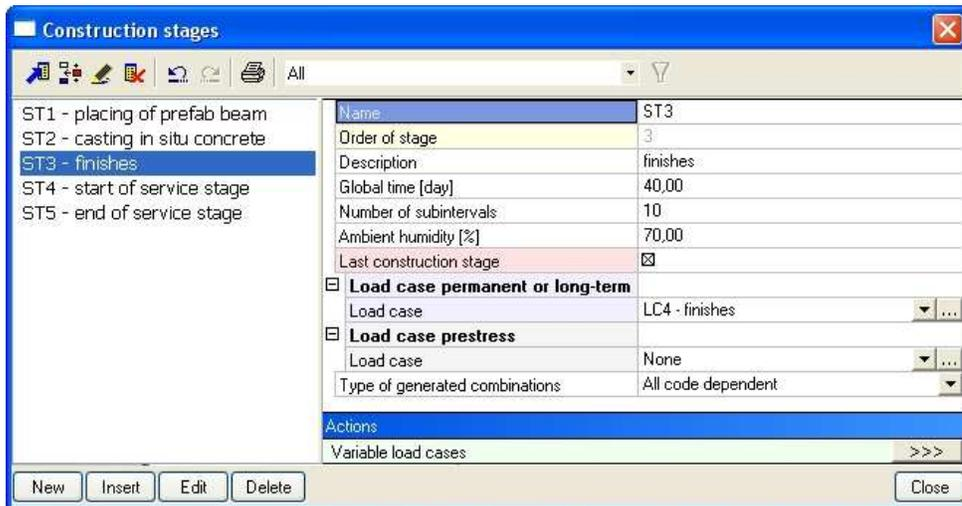
Note that stage 3 is the last construction stage. This means that after this stage, it is allowed to add service loads of type long term variable.
