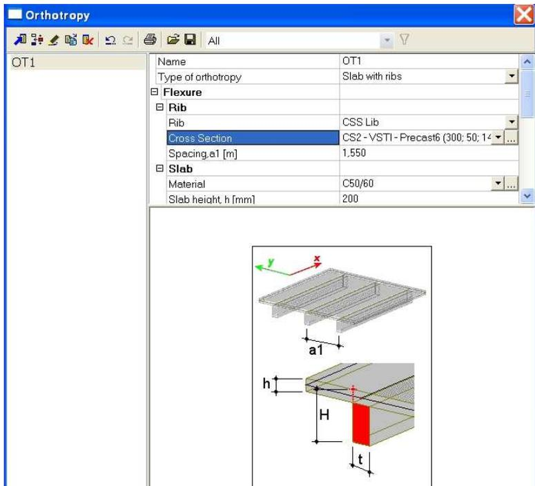
The prefabplate will be modelled with a total width of 15m and a span of 30m. The supports have to be applied as nodal supports on the beam edges.
