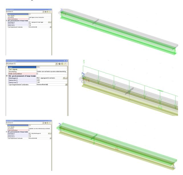
The indication of the construction stage in which the phase change of the cross-section occurs is done in the properties of the member:
