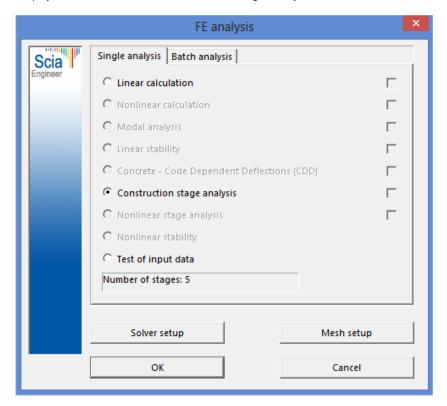
Next to the results for every load case individually, also the results for the summation of the different linear load cases can be viewed. For every stage, automatically an envelope combination and a class is created which contains the summation of the results in that stage including the history of all previous stages.
