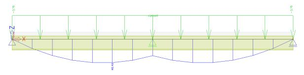
Class stage 3: By removing the support, the final moment line is that of a simply supported beam under self weight of both the steel(applied in stage 1) and the concrete (applied in stage 2).
