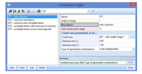
After definition of the stages, the user should indicate which members or supports shall be added or removed in every stage.
