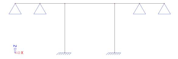
LC 2: the introduction of the beam element causes a moment in the beam, but also in the columns, because of the fixed connection.
