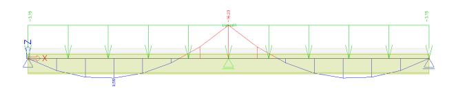
BG3: effect of removal of the support (notice that this is the moment line corresponding to the application of the inverse of the reaction force of the removed support)
