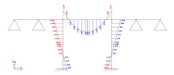
LC3: In this load case the side beams are added. Notice the extra moments. Since the end beams are connected rigidly with the existing frame, the moment in the end beams (1,07 kNm) will be equal to the sum of the moment in the middle beam (-0,39 kNm) and the column (-0,68 kNm)..
