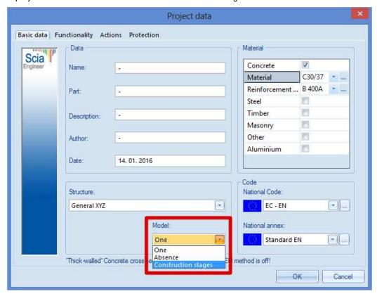
The model will be built up of construction stages, instead of one model.
