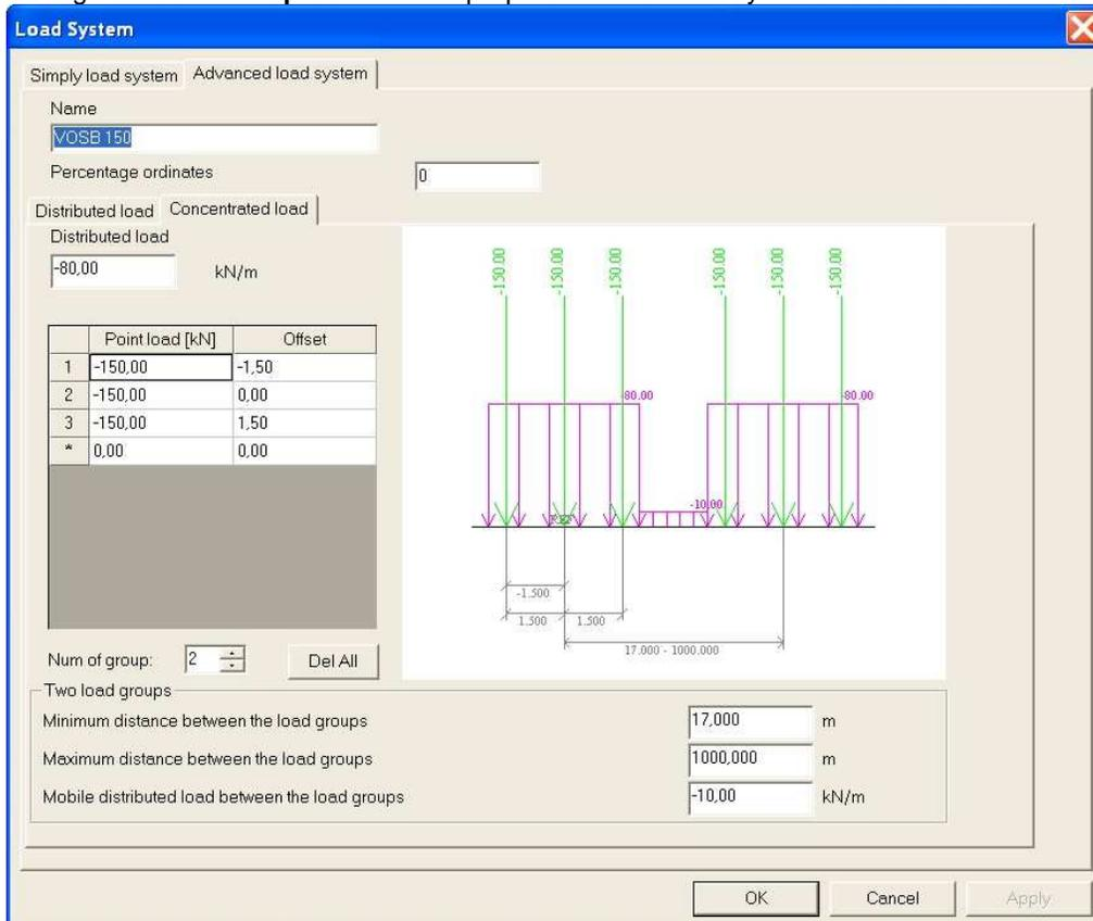
The load system consists of 2 groups of three point loads and a divided load. The point loads have a value of 150 kN and a mutual distance 1.5m. The divided load has a value of 80 kN/m.
