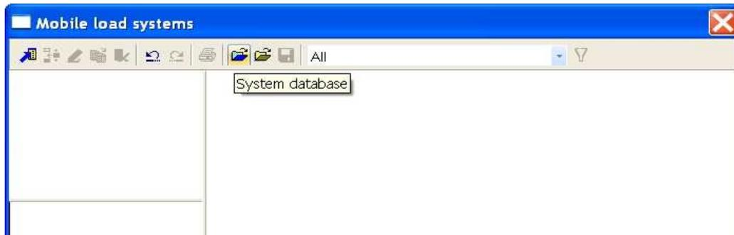
Through the button System database
