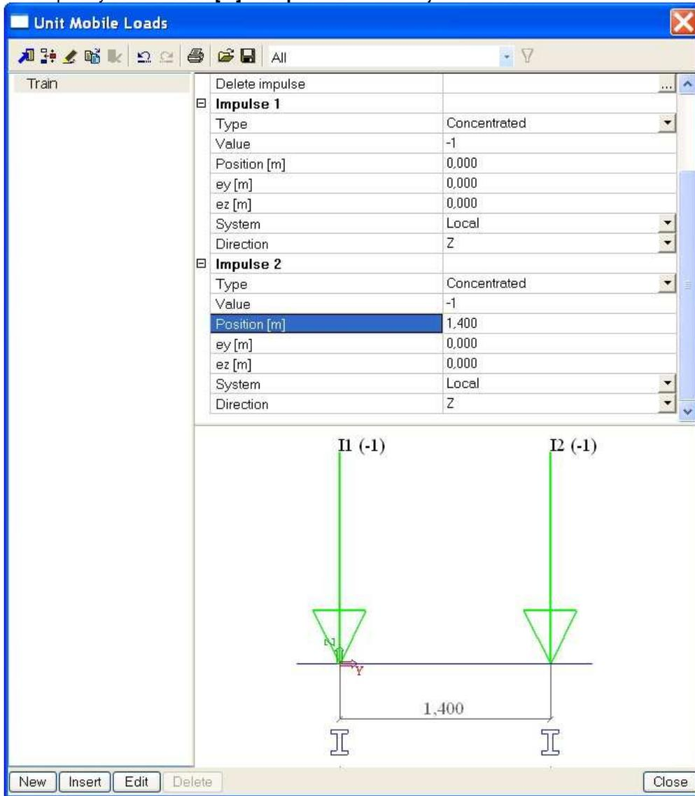
Both impulses are displayed on the bridge deck:
