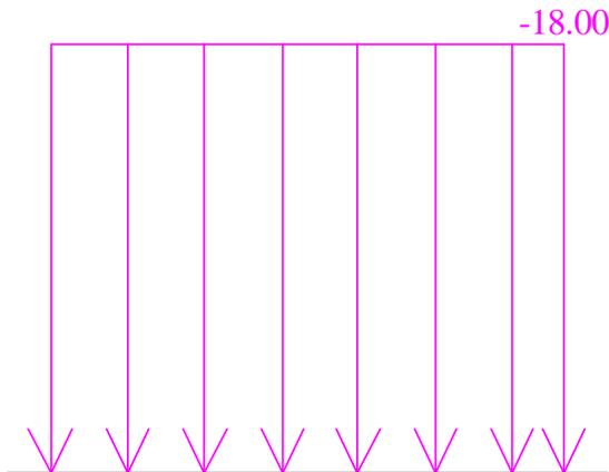
When entering a Single Load system, you have the possibility to mark the option **Neglect point load with opposite influence**. If this option is activated, the complete concentrated load, which lies in the negative area of the influence line, will be taken in account in the calculation. By activating this option, the found maximum will be reduced.
