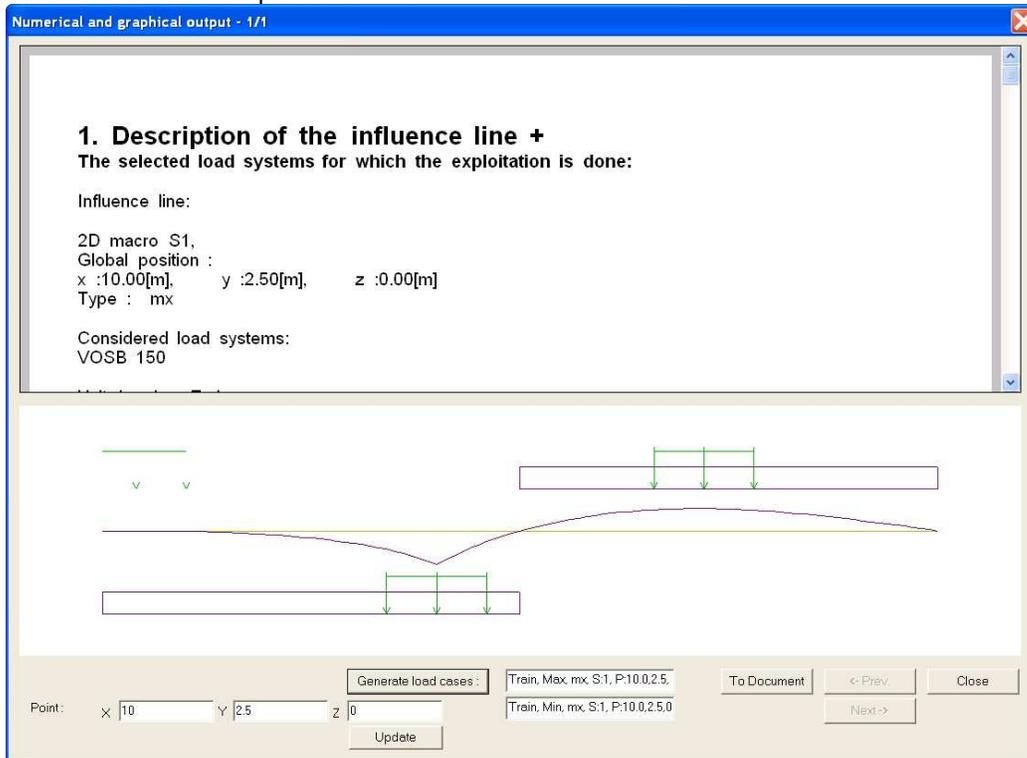
Through **Generate Load Cases** the load cases are generated.
