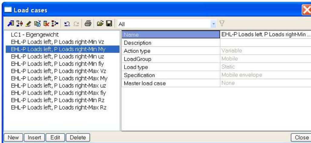
The load cases have 'Mobile envelope' as a description and are in an exclusive load group. If required, the load group can be adjusted to set a Load type according to EC1991.
