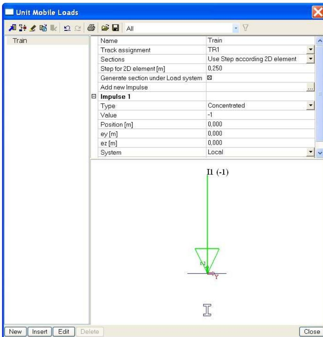
Now the unit load consists of 1 concentrated load. To show both rails of the train track, a second impulse is added through the option **Add new impulse ...**.
