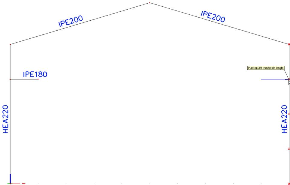
To be able to get the full hall, the option
