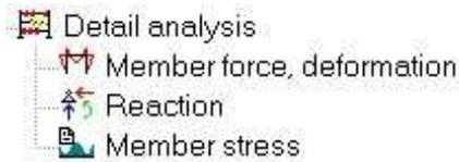
With the **Detailed Analysis**, the load systems can be linked to the unit load. For every desired position on the structure, between all the selected tracks, SCIA Engineer determines the system that is most adverse for the chosen design parameter.
