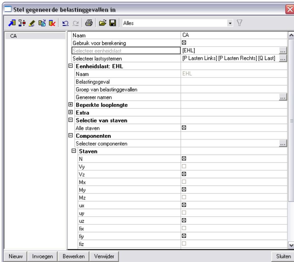
First of all you have to indicate which unit loads and which load systems have to be taken into account. In this example three imported load systems are selected.
