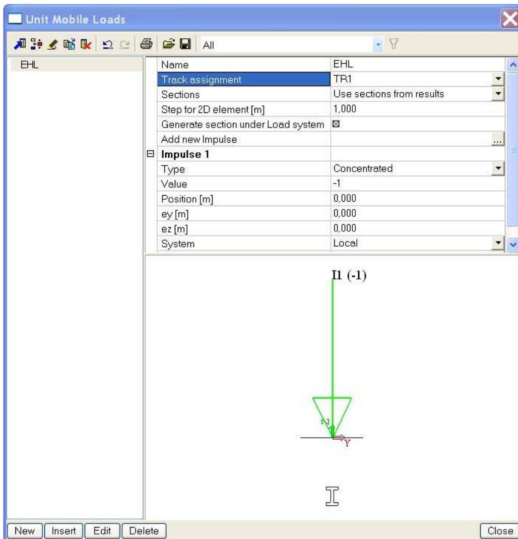
Through the option **Track assignment** you can indicate on which track the unit load needs to appear.
