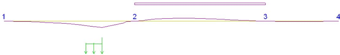
An influence line for a point of the construction is the representation of the amplitude of the design parameter in the point, if the unit load is moving across the structure. By placing the divided load on the places where the influence line has the same sign, an extreme result is obtained. In this example the moment  $M_y$  on 24m reaches a minimal value **-622.15 kNm** if the divided load is placed in the second field.
