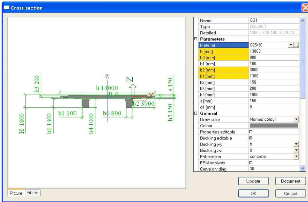
The construction can be inserted as 3 horizontal beams through Beam, at which the begin node is imposed hinged and the other nodes are rolled.
