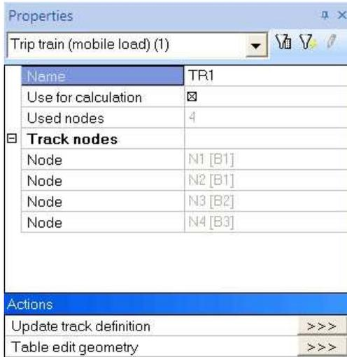
After defining the track, a unit load can be inserted through the menu
