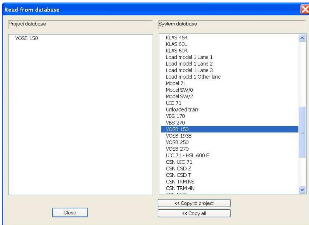
With the button
