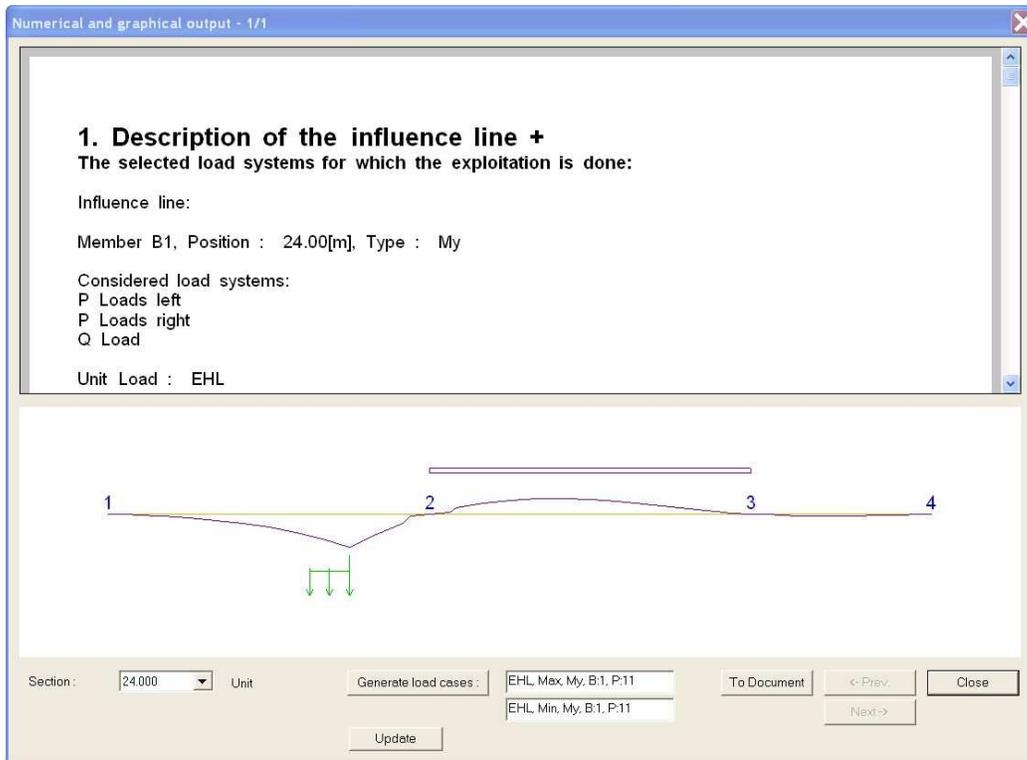
Through the button **Generate Load Cases** two load cases are generated, one for the minimal My on 24m and one for the maximal My on 24m. The parameter B indicates the member, parameter P the position on the member.
