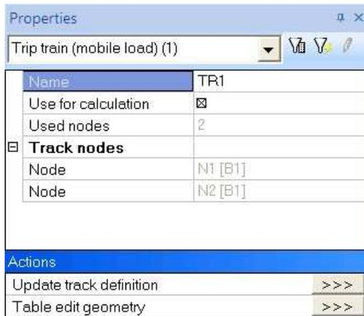
The option **Use for calculation** shows that this track is taken into account in the calculation. If more tracks are defined, this is way can be used to show which tracks really have to be calculated. The action **Update track definition** allows generating the imported track again if e.g. the coordinates of a node were adapted. That way the track doesn't have to be imported again after an adjustment of the geometry.
