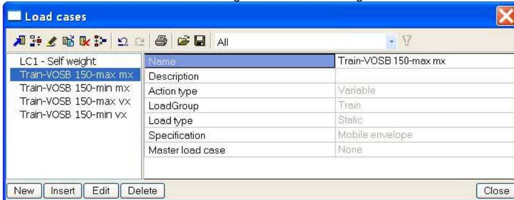
The load cases have Mobile envelope as a description and are in an exclusive load group. The load group can be adjusted if required to set a Load type according to EC1991.
