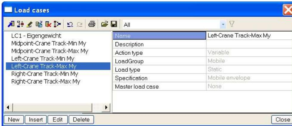
The load cases have Mobile envelope as a description and are in an exclusive load group. If required, the load group can be adjusted, e.g. to set a moment factor according to NEN or a Load Type according to EC1991.
