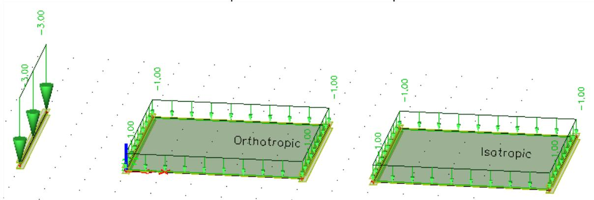
As the plates are 6m x 6m, and the surface loads are 1kN/m<sup>2</sup>, the load transferred to the beams should be around 3kN/m.
