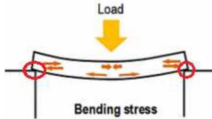
As a result, the supports force the elongation at the bottom fibre to be zero by means of a reaction force. This can also be seen in the results.
