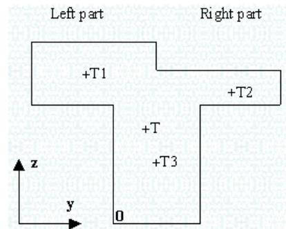
The internal forces in the plate can be found by a section on the middle of the plate, over the width. Then the averaged results over this section can be found.
