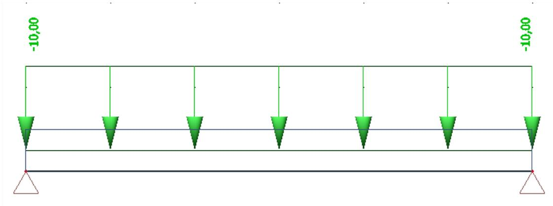
As you can see, the line load is inputted on the beam and follows the eccentricity of the beam. The supports are in the nodes, which are positioned eccentrically from the neutral line of the beam.
