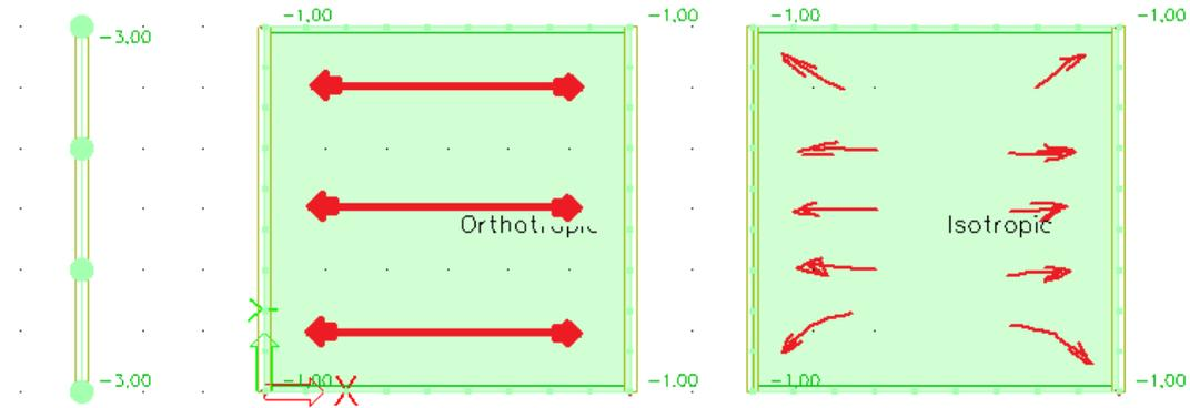
This effect would even become more dominant if the stiffnesses are higher. To show this, the thickness is doubled in both the orthotropic and isotropic plate. To do this, the OT1 setting is changed, and the properties of the isotropic plate are changed.
