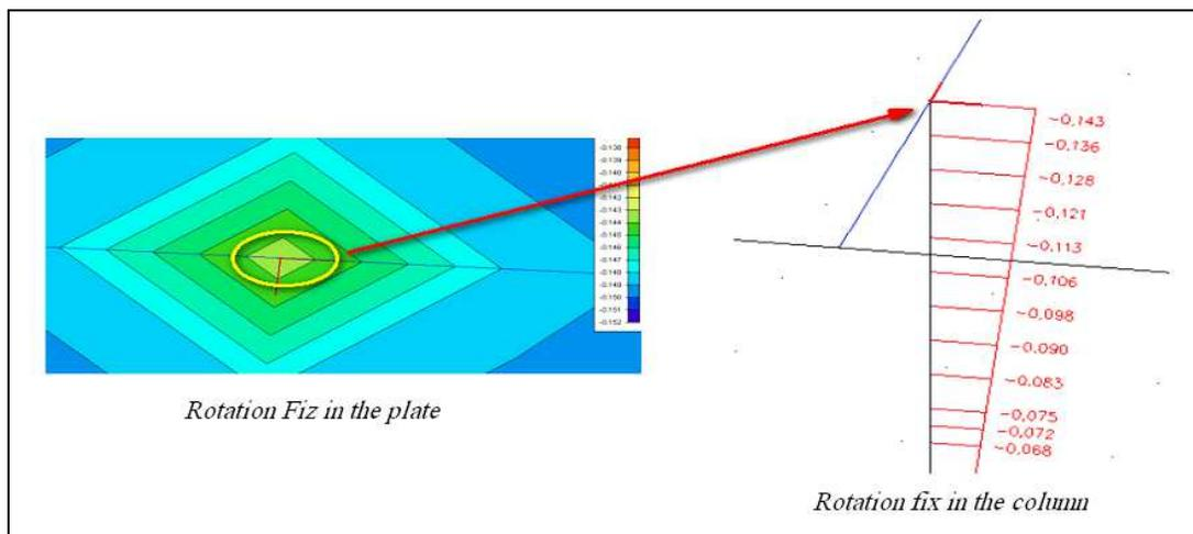
Applying two crossing dummy-members at the connections is a way to get a correct approach of the reality. These are attached to the plate by means of internal edges. This way, the small beams will take the rotation of the plate on themselves, so the plate has a stiffness around the Z-axis. In this case, the large deformations at the edges will be gone.
