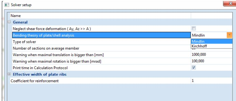
This option is only in relation with 2D elements. Specifically for beams, the shear force deformation can be taken into account or not by means of the option **Neglect shear force deformation ( $A_y, A_z \gg A$ )**.
