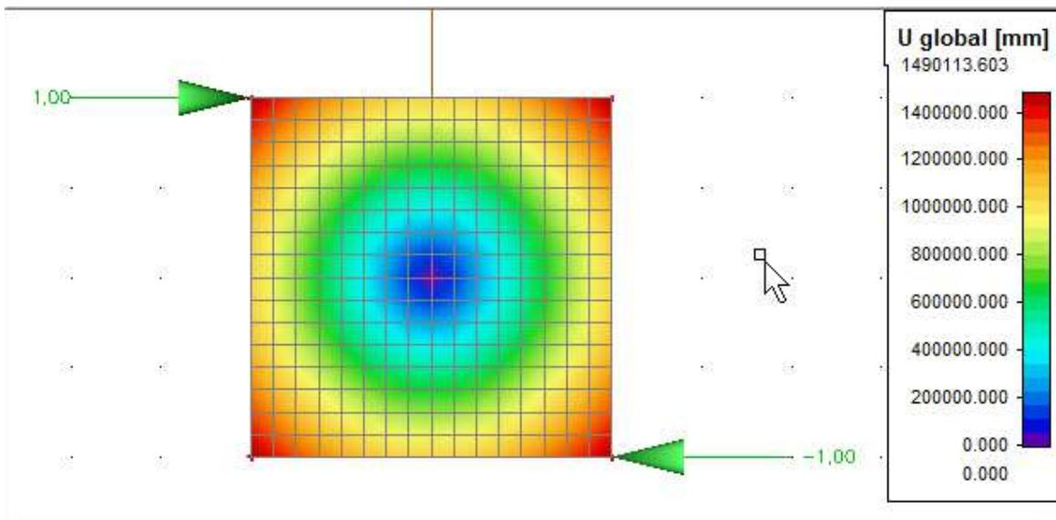
This phenomenon can be ascribed to the fact that the plate has no rotational stiffness around the Z-axis. 'Energyless' deformation occurs, which means that the plate does not know any resistance against the deformation  $\varphi_z$ .
