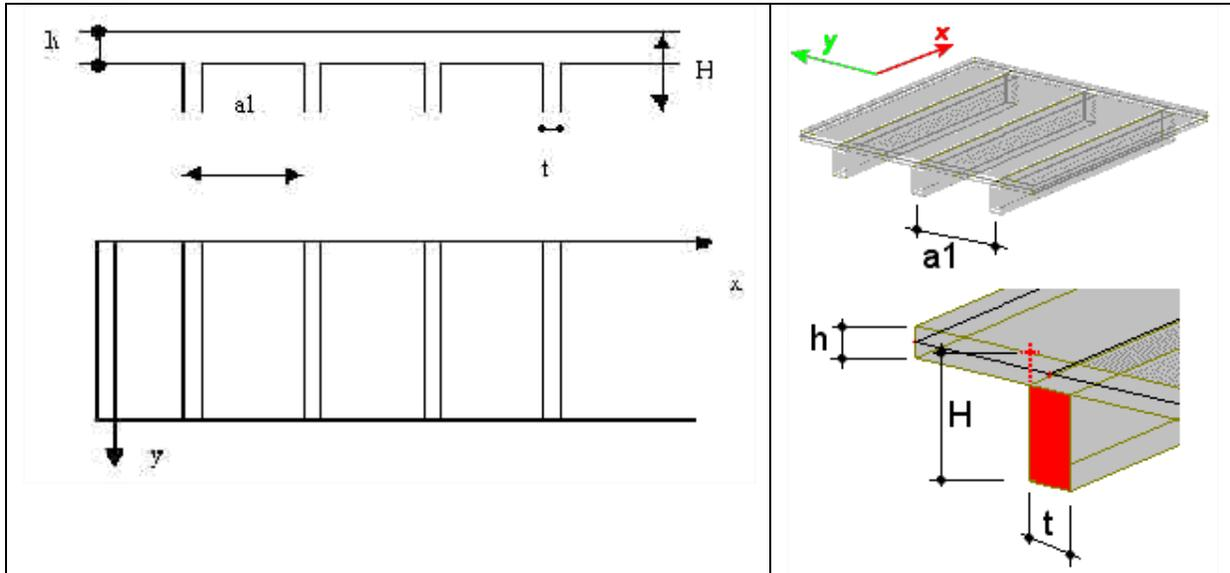
The user must select the rib from the library and input the rib spacing and slab height..
