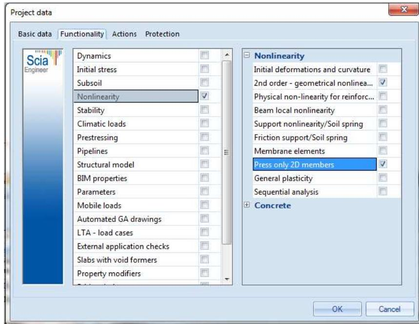
With this option, tension in 2D elements can be automatically eliminated. This is mostly used for masonry elements. When using this functionality, it is advised to adjust some parameters to smoothen the calculation. This will be treated in the next examples.
