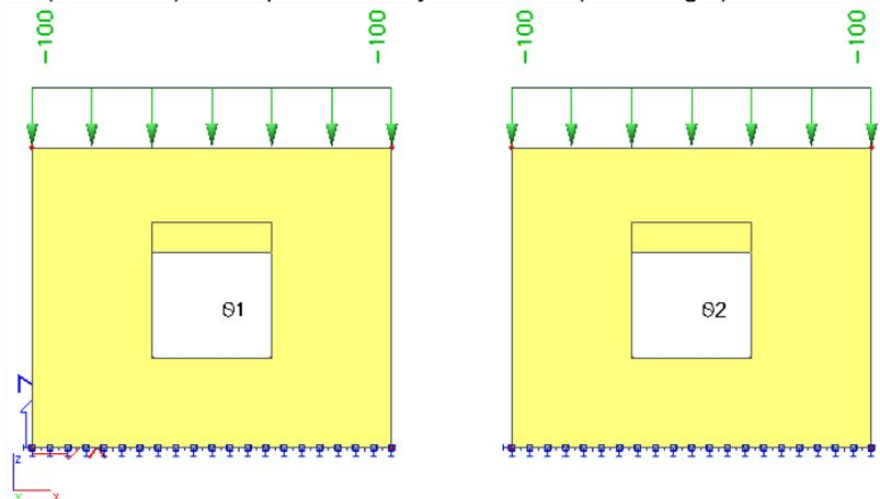
Since a pressure only wall cannot take any tension, there are beams added over the opening to take the tension in that position.
