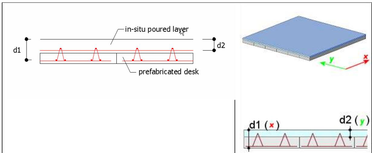
The user must input the effective heights and reduction coefficients:
