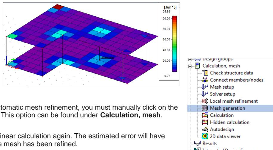
4. To perform the automatic mesh refinement, you must manually click on the mesh generation. This option can be found under **Calculation, mesh**.
