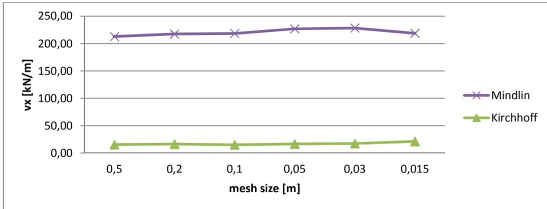
In this case, calculating with Kirchhoff is a better option, because Mindlin does not give good results, unless you would use an unrealistic small mesh along the border.
