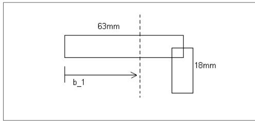
$$b_1 = \frac{(63 \times 2) \times 63 / 2 + (18 \times 2) \times 63}{(63 \times 2) + (18 \times 2)} = 38,5 \text{ mm}$$
