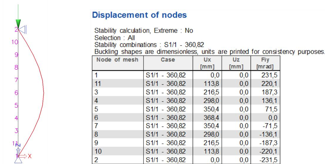
Using for example an Excel worksheet, the buckling shape can be approximated by a 4<sup>th</sup> grade polynomial.
