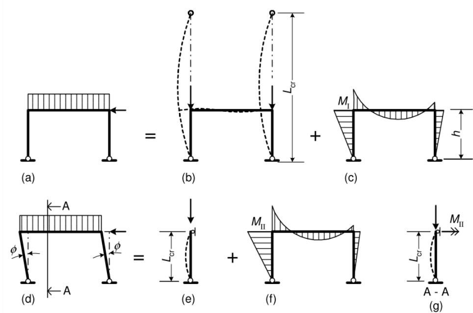
The equivalent column method is illustrated by (a), (b) and (c), where (a) is system and load, (b) is equivalent column length and (c) is the first order moment.
