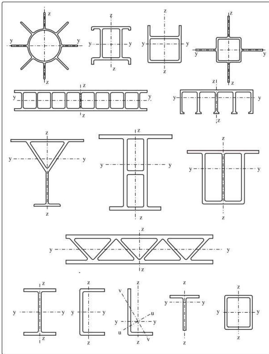
SCIA Engineer will use the axes y-y and z-z respectively for the major and minor principal axes of the cross section.
