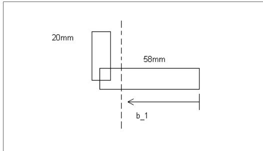
$$b_1 = \frac{(58 \times 2) \times 58 / 2 + (20 \times 2) \times 58}{(58 \times 2) + (20 \times 2)} = 36,44 \text{ mm}$$
