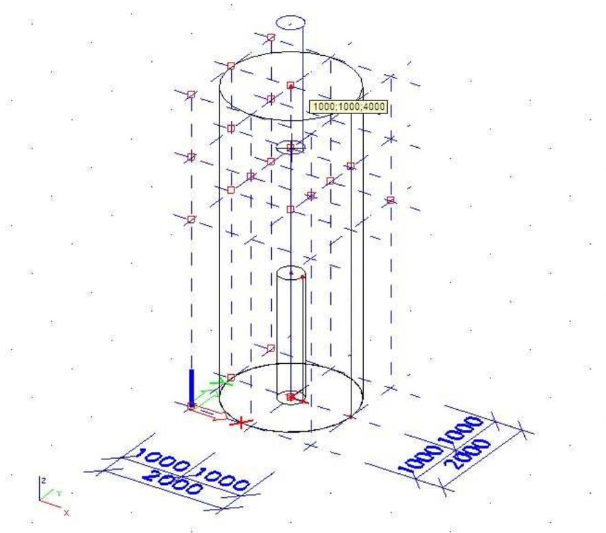
14. Now the cylinder has to be rotated. This is done by using the command rotate
