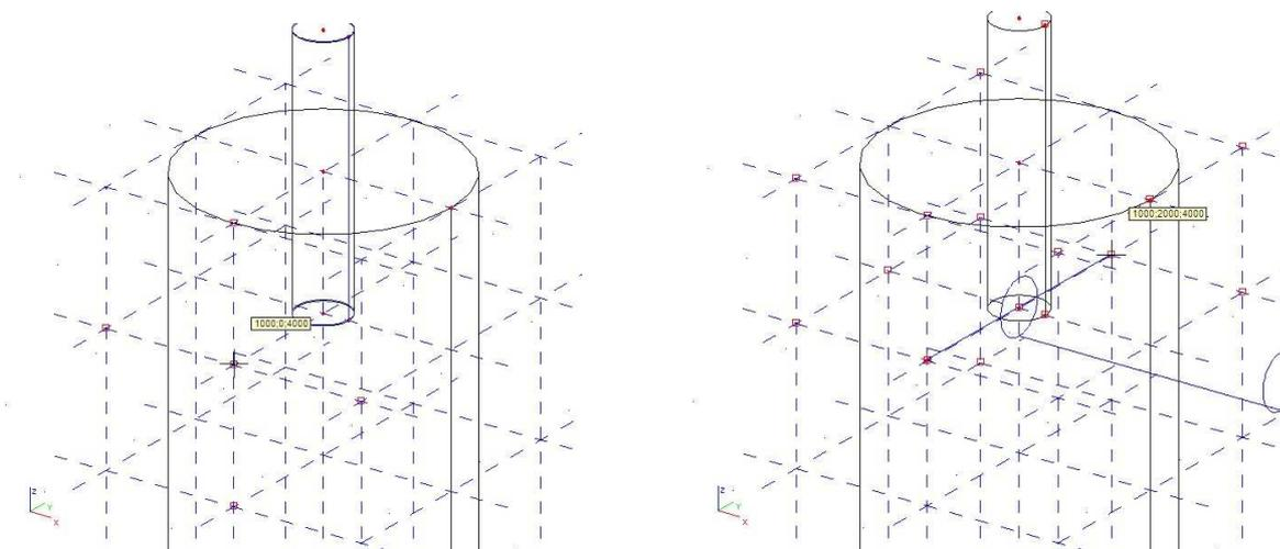
20. The cylinder was rotated on the axis with an angle of 90°, defined by the user.
